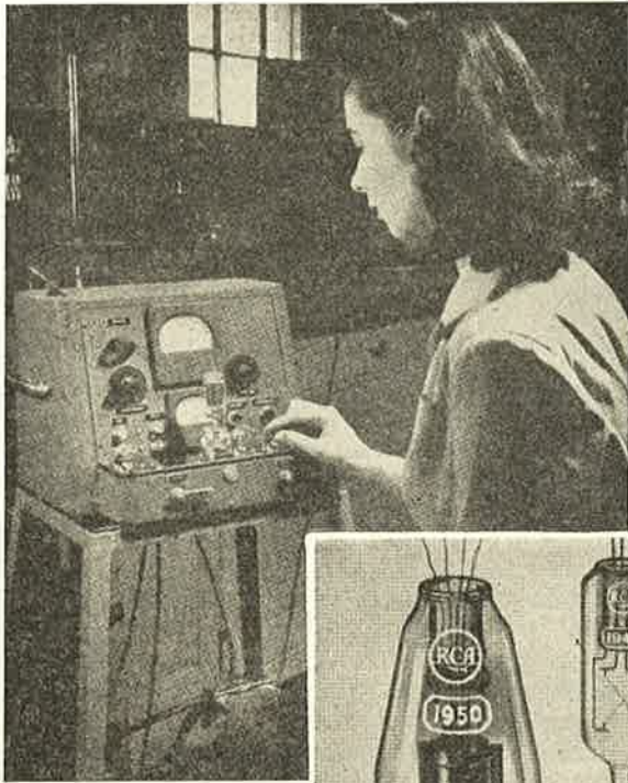
Fig. 1—Portable, easily operated, commercial leak detection equipment (RCA model 722-SS) using hydrogen-sensitive ionization tube.
