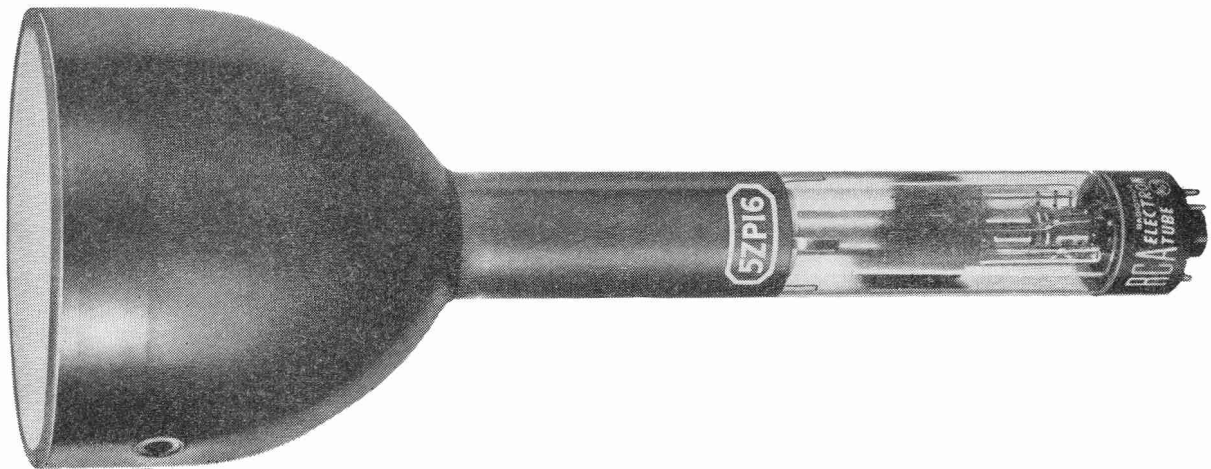
Fig. 1.—A Typical Five-Inch Flying-Spot Scanning Tube, the 5ZP16.
