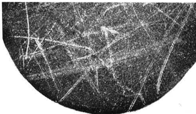
Figure 1.—Section of part of an uncarburized thoriated tungsten wire. (Cf. Figure 2.)
