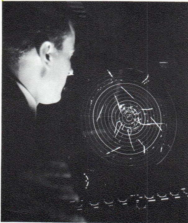
Observation on a TV screen of a PPI aerial picture converted by means of a scan conversion tube, the remanence of which allows visual aircraft tracking.
