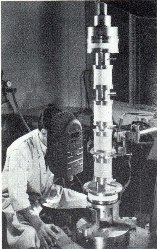
"Argonac" welding of a F2008 klystron body on an automatic machine.
