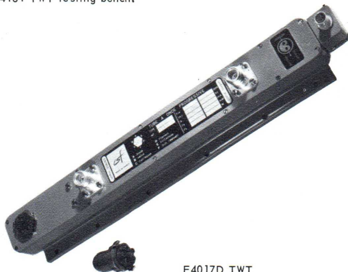
F4017D TWT cooled by conduction
