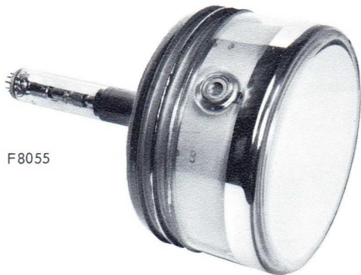
The "Cyrano" radar set-up on the "Mirage III" airplane is fitted out with a CSF direct view storage tube.
