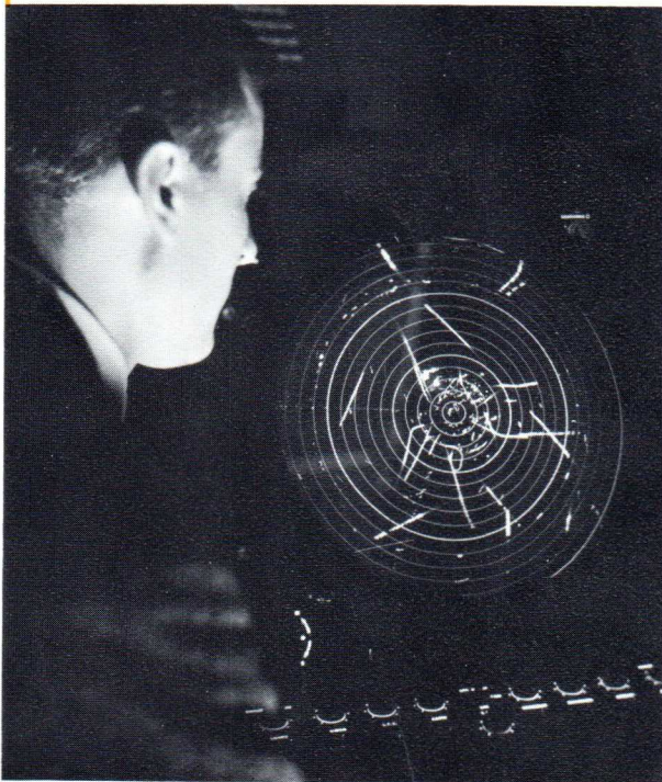
Observation on a TV screen of a PPI aerial picture converted by means of a scan conversion tube, the remanence of which allows visual aircraft tracking.
