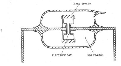
At low voltages the gap is a good insulator with a very low leakage current. As the voltage to the spark gap increases an avalanche effect is created until a point
