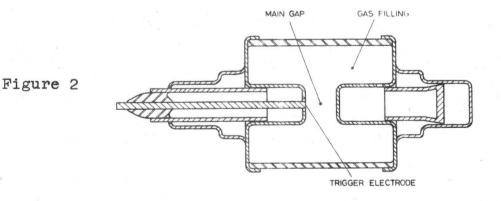
it possible to establish an arc at gap voltages below the breakdown value. Over a wide range of gap voltage a low-energy pulse applied to the third trigger electrode produces a small arc which transfers rapidly to the main
