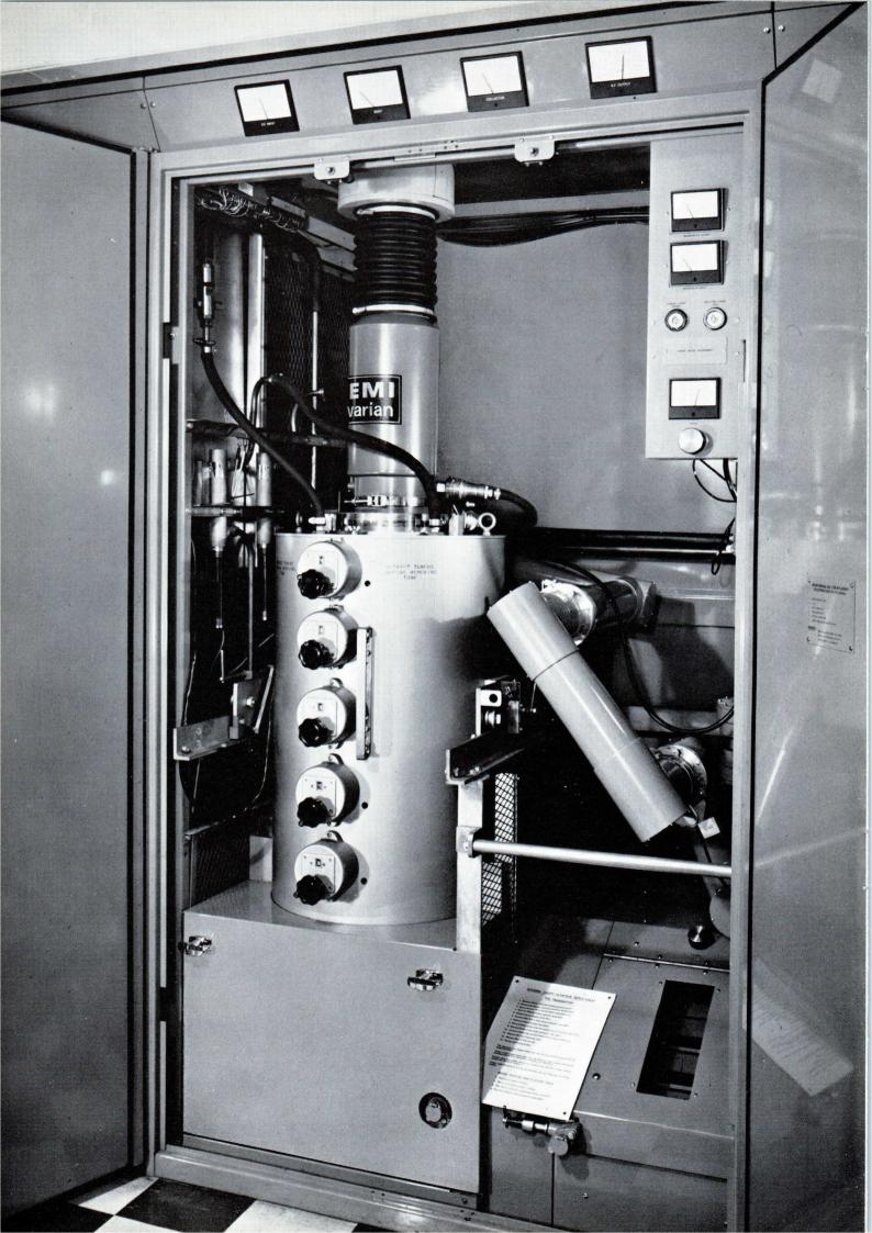
With the cavities part of the vacuum envelope many ceramic to metal seals and external sliding contacts are eliminated. The integral cavity klystron is therefore rugged and reliable.
