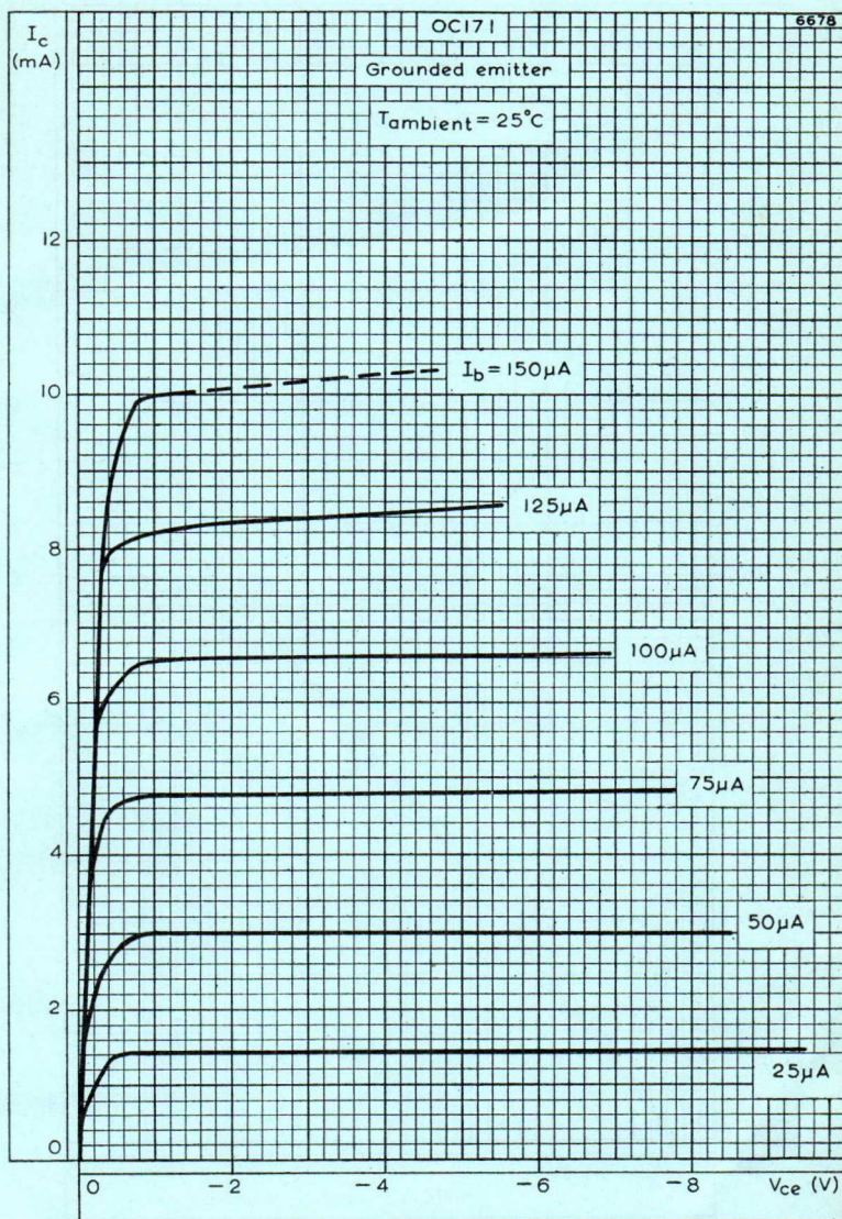
OUTPUT CHARACTERISTIC. GROUNDING Emitter
