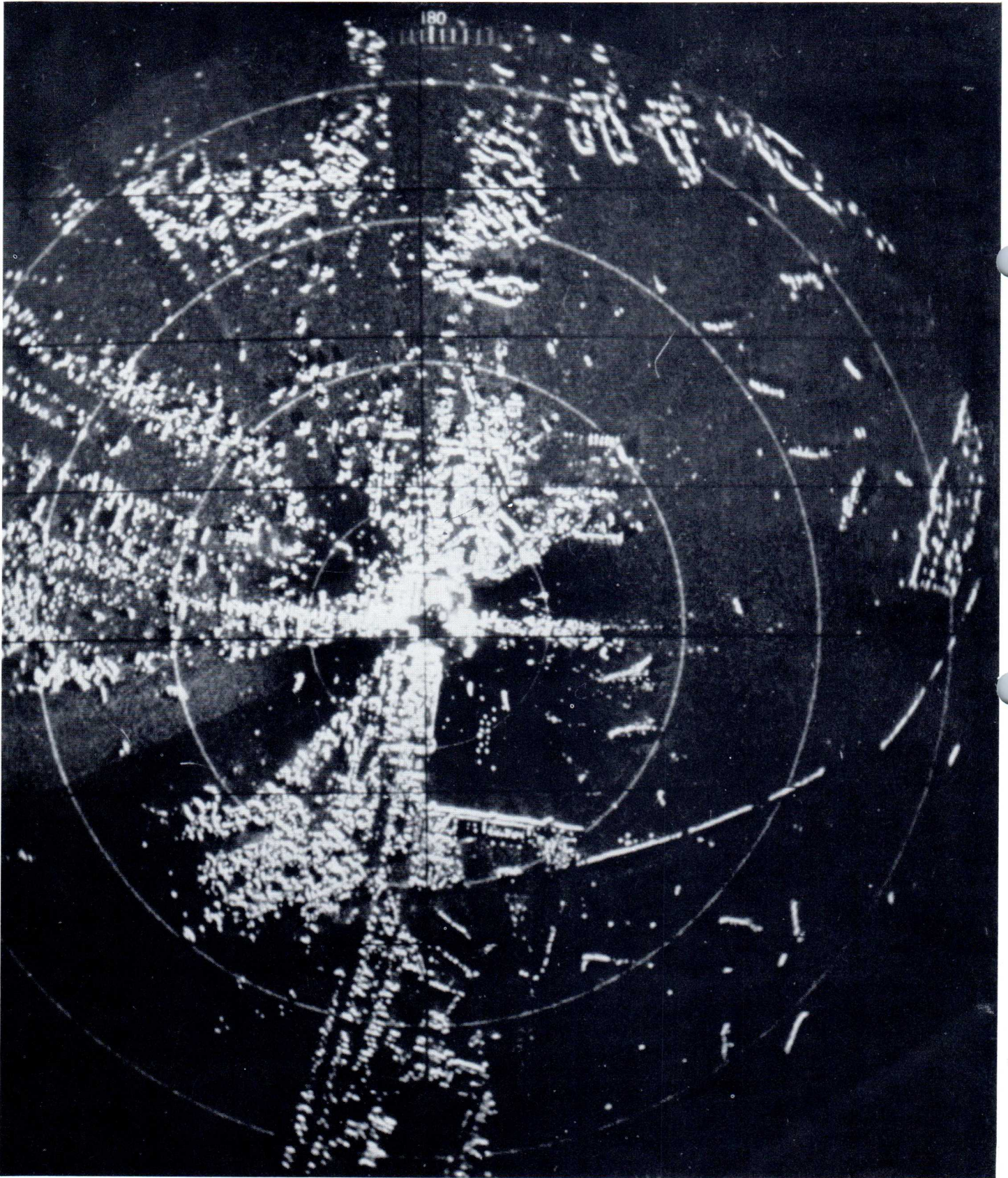
RADAR IMAGE OF BALANCED BEAUTY of 8.6mm wave High-Resolution Radar CPH-1 showing Yokohama Harbor, radar range 2km
