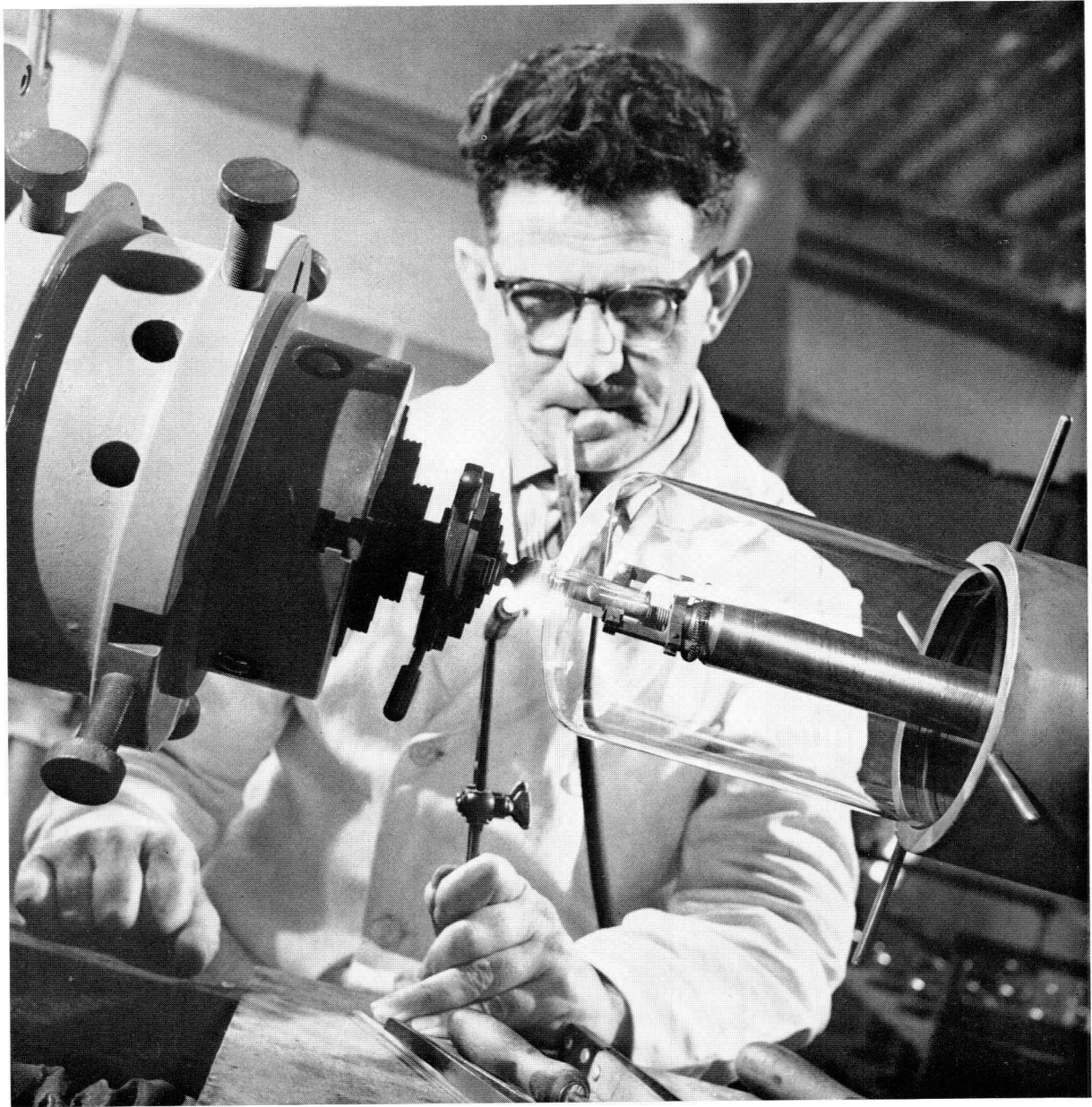
The anode connection is sealed to the tube envelope
