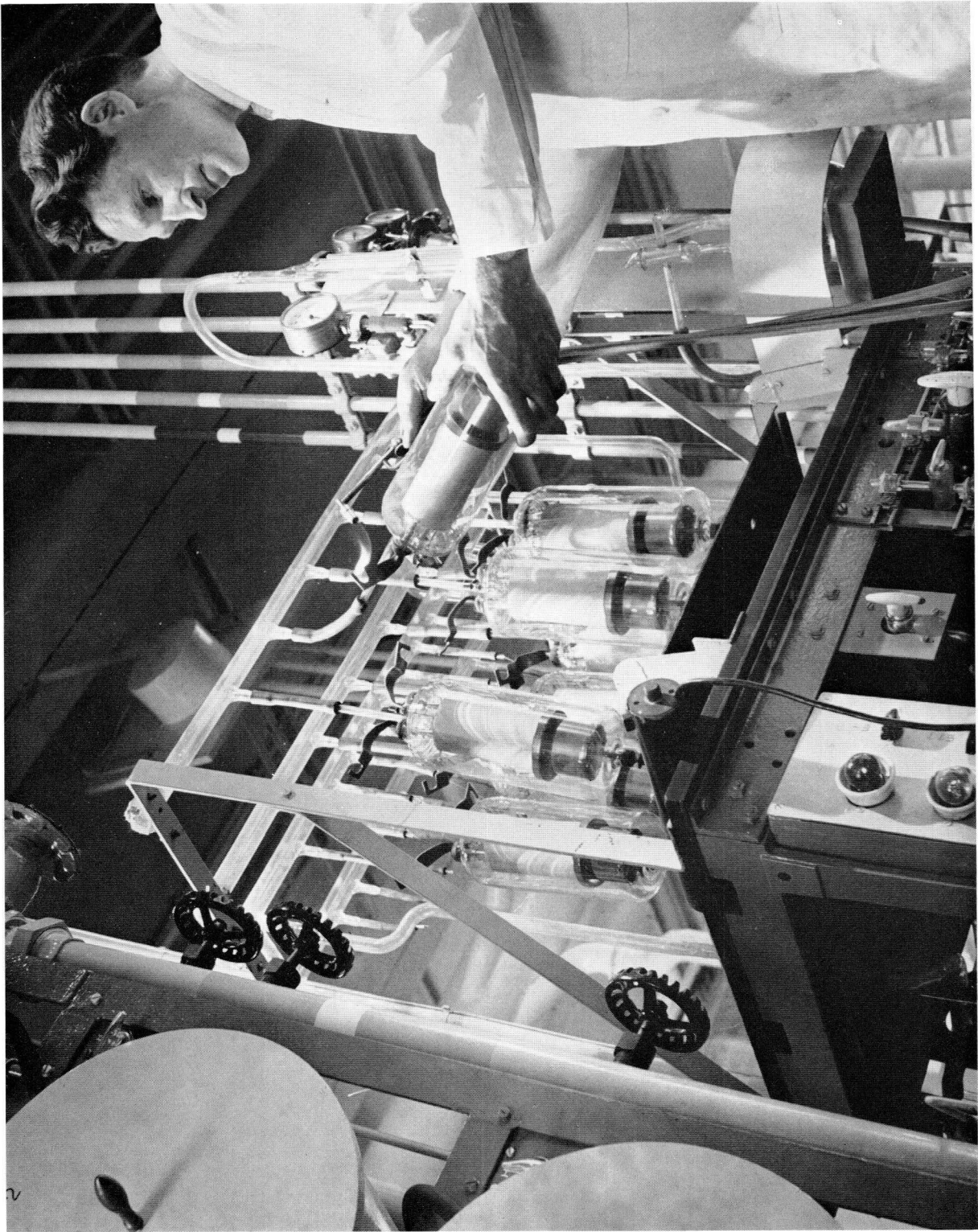
Before being evacuated the thyratrons are prepumped
