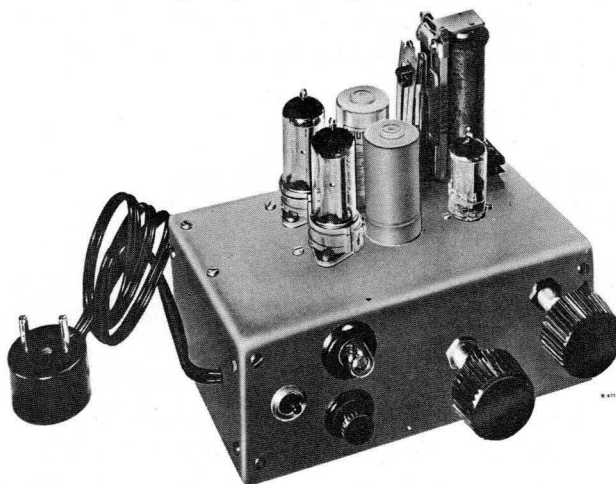
Fig. 3.3. Experimental unit using the circuit of Fig. 3.2.
