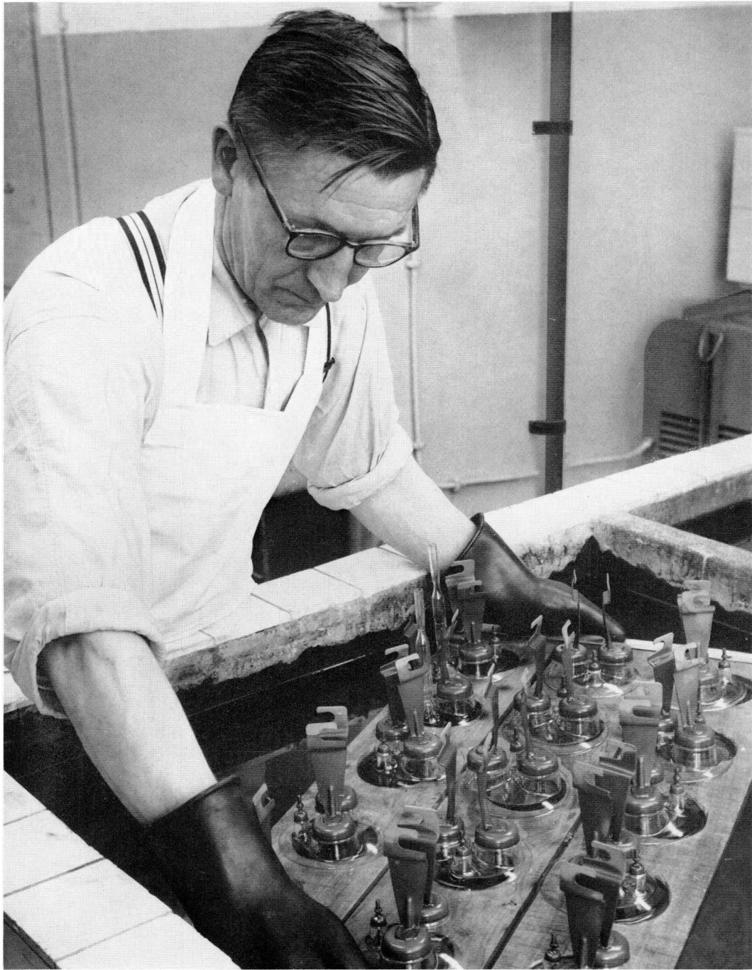
A batch of tube bases is cleaned and degreased
