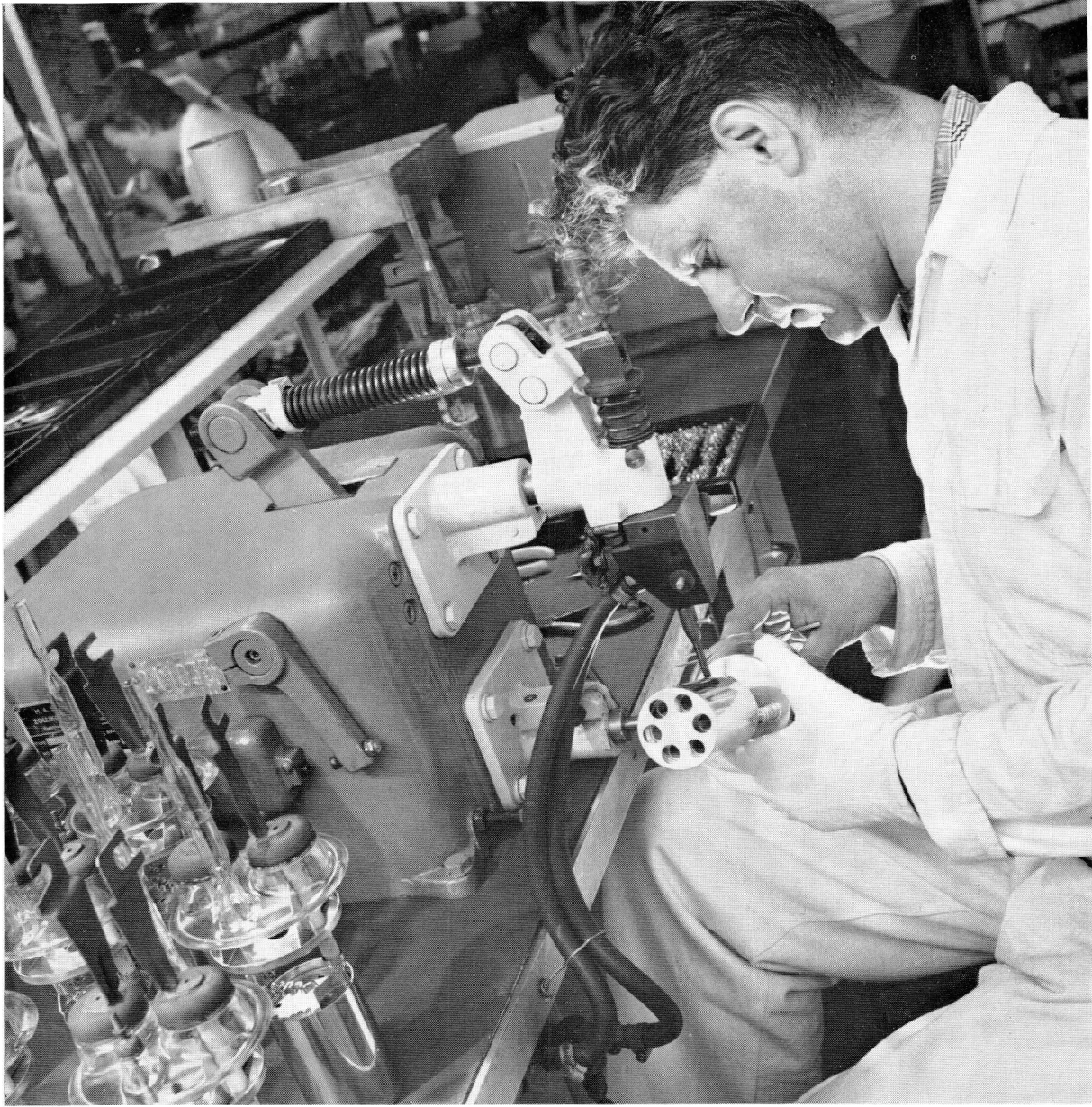
The cathode assembly is spot-welded to the tube base
