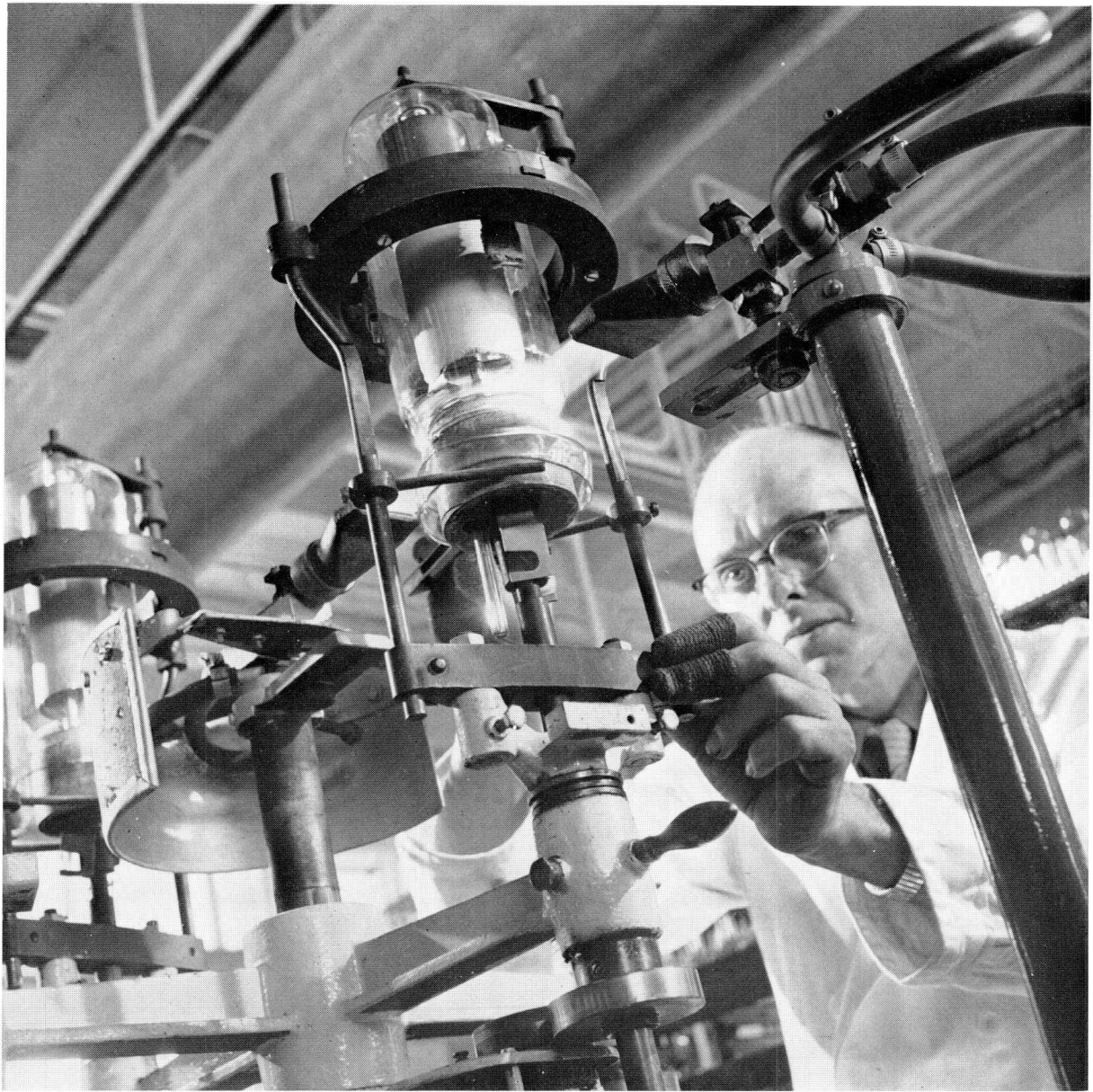
The tube base is sealed to the envelope
