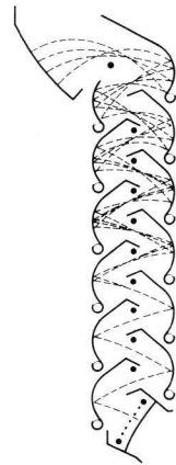
Fig. 4.13. Construction of the multiplier of a fast photomultiplier: (a) detail of dynodes, (b) overall view.
