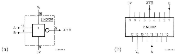
Fig. 2-31 2.NOR61 as a dual-input NOR gate: (a) circuit diagram, (b) wiring diagram.
