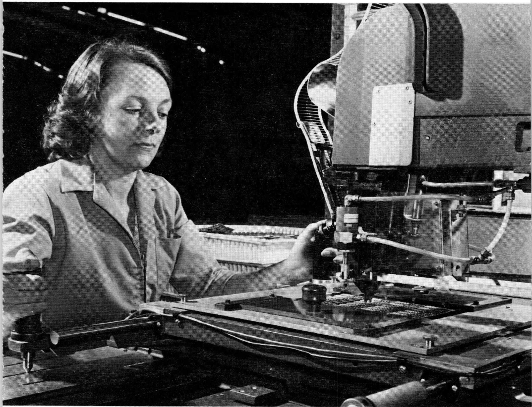
Automatic assembling of resistors on NORbit p.c. boards.
