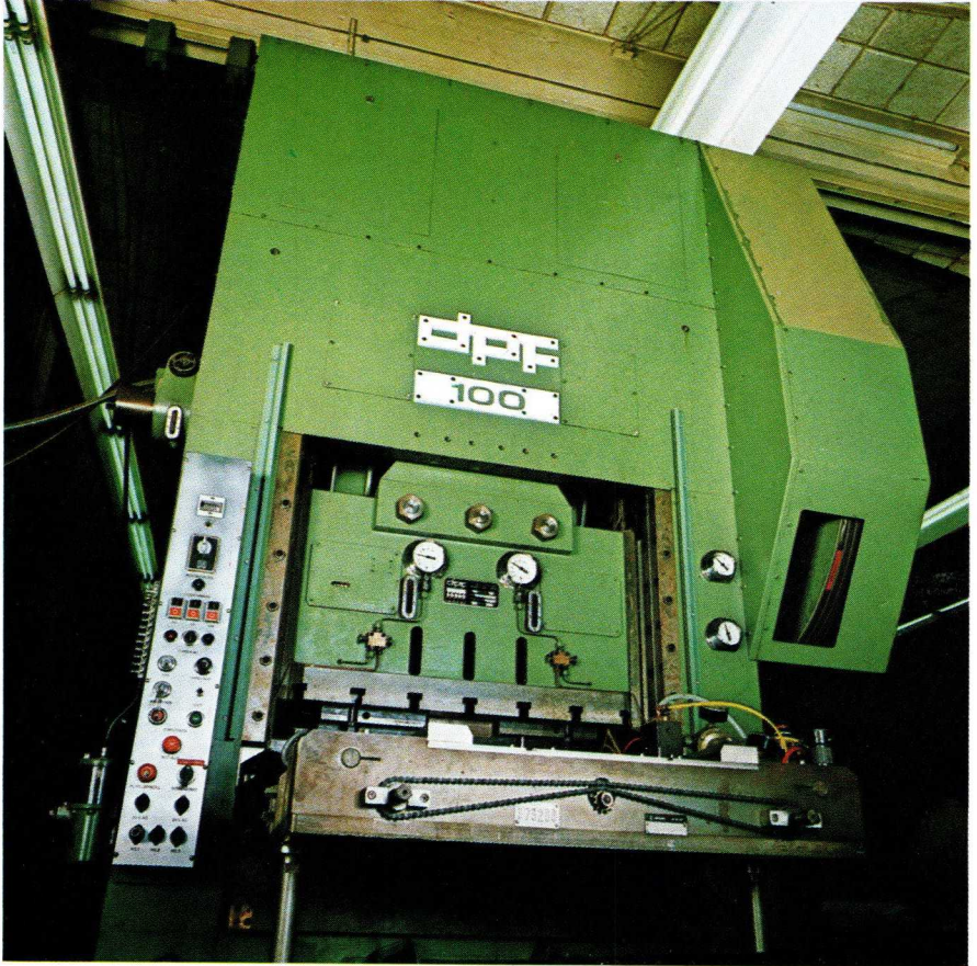
This 100-ton press for p.c. board manufacture is driven by a variable-speed 10 h.p. motor which is supplied from a 12 kVA three-phase inverter of the type described in Section 4.6.3.
