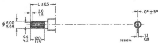
Fig. 3. Plastic spindles in fully counter clockwise position ("off" position for rotary switches)
