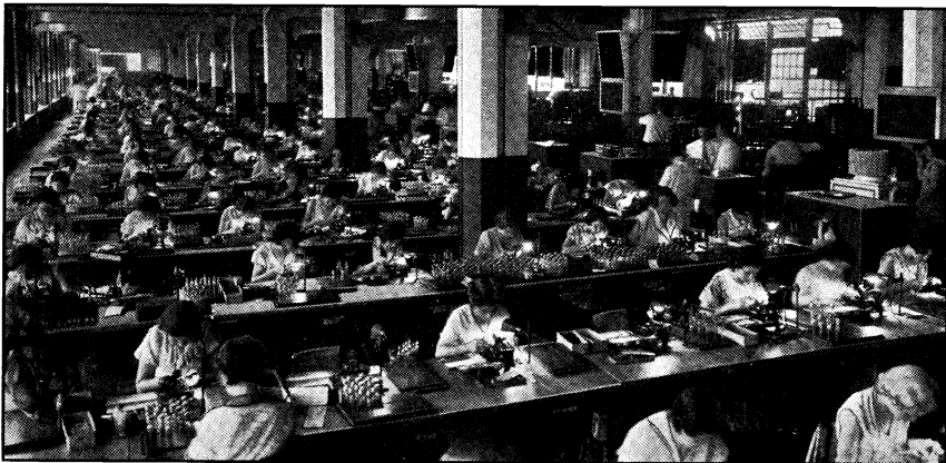
Assembling Radio Tubes
