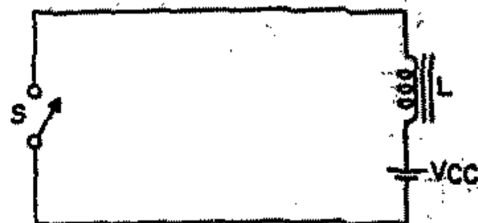
Fig. 85—Simplest form of deflection circuit.
