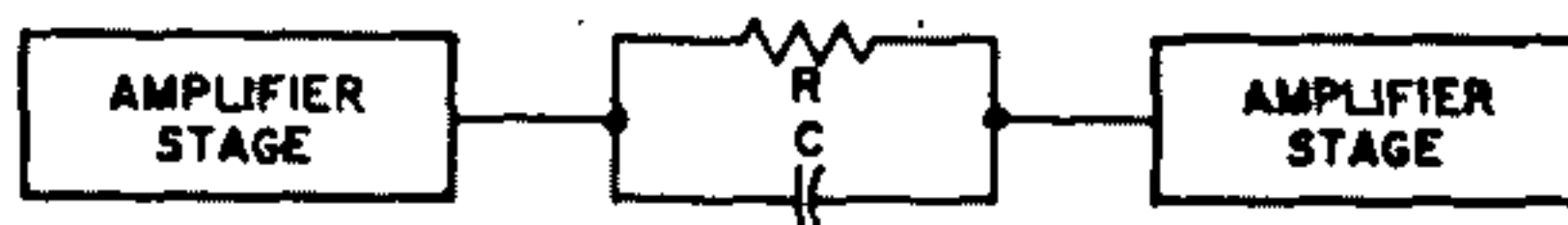
Fig. 54—Simple RC frequency-compensation network.
