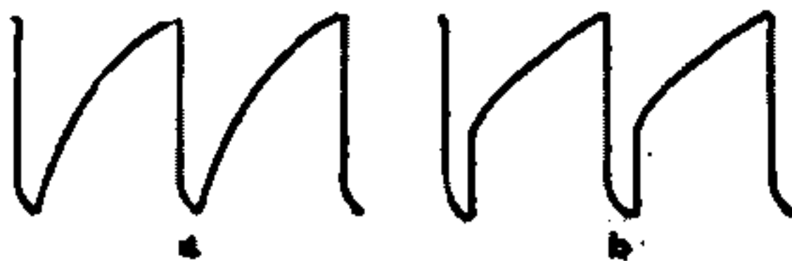
Fig. 91—Waveforms showing effect of R_2 in Fig. 90.
