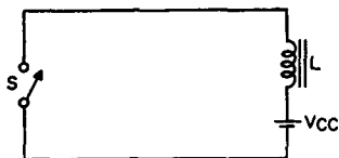
Fig. 85—Simplest form of deflection circuit.
