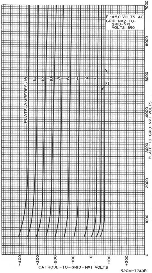
Fig. 15 - Average Constant-Current Characteristics for Cathode-Drive Operation of Type 6166-A/7007.
