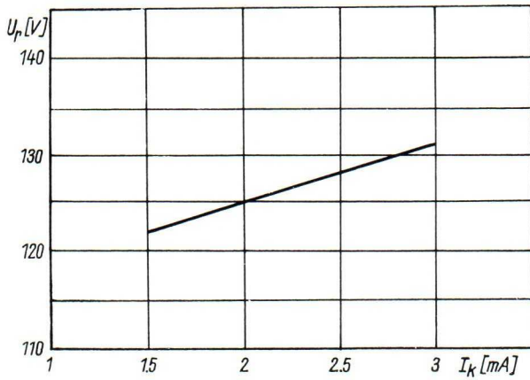
Running Voltage as a Function of Cathode Current (also applicable to Type Z 561 M)
