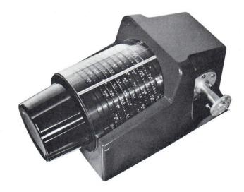
Attenuators can be supplied with attenuation ranges greater than 60 dB. They can also be furnished in a combination with a rotary phase-changer unit. These units are usually coupled at the circular waveguide section to minimize mismatch errors at low attenuation settings.
