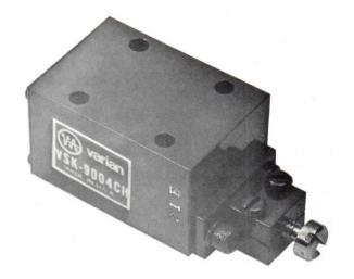
Cooling is achieved by attaching the oscillator to a heat sink which maintains the oscillator temperature at  $50^{\circ}\,\mathrm{C}$  or less.
