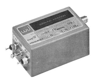
WJ-2804-10 is a voltage-tuned transistor oscillator designed to provide fundamental microwave power over the 2 to 4 GHz range. Varactor tuning ensures a high tuning input impedance characteristic for the device. Two transistors in a push-pull configuration provide superior out-of-band harmonics rejection. Since the device is a fundamental oscillator, no inband harmonics are exhibited.
