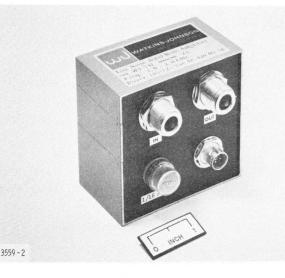
Modular construction ensures high reliability under adverse operating conditions. The microstripline circuit configuration employs integrated circuit biasing and bypass modules for consistently high performance. The overall design of the WJ-741 is consistent with the general requirements of MIL-E-16400 and MIL-E-5400, class II. Since the amplifier is tested and set for operation prior to shipment, no adjustments are necessary by the user.
