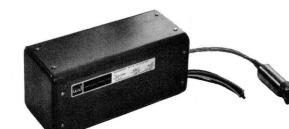
The WJ-2018-51 is a magnetically shielded and RFI shielded voltage tunable oscillator utilizing a bifilar (dual helix) and a permanent-magnet focusing system. Unsaturated magnetic shielding reduces the magnetic field strength along the outside of the housing. RFI
