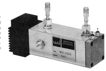
The WJ-4523 cavity amplifier is a compact modular amplifier readily adaptable to airborne or ground support telemetry and communications systems. It is an optimum combination of the tube configuration with the associated rf circuit. Maximum efficiency and rf output from a very small package are outstanding features offered by this amplifier. Tuning can be accomplished with a minimum of test equipment.
