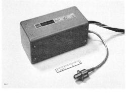
in frequency diversity transmitters (as master oscillator), and in ECM equipment. Fine grain variation of frequency versus voltage is extremely low. The WJ-2033-1 delivers smooth power output over the band with low operating cathode current. Power can be modulated and leveled with either grid or anode circuits. All voltages are isolated from housing and RF output connector for maximum
