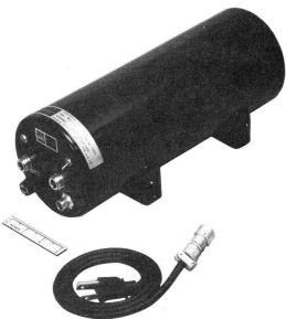
The WJ-399-2 is a higher output power version of the WJ-399 with a typical output power of 80 mW. Like its lower-power predecessors, the WJ-399-2 is completely self-contained, adjustment-free, and requires only a 115-volt ac line-voltage input (48 to 420 Hz).
