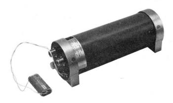
operation. It may be operated in any orientation. Rugged construction of the tube, magnet, and power supply assembly ensures reliable operation under vibrational forces of 10 g, at frequencies up to 500 Hz. Full specifications are met over the operating temperature range of -54 °C to +71 °C. The environmental characteristics of the WJ-458 meet or exceed the corresponding requirements of MIL-E-5400, class 2 specification.
