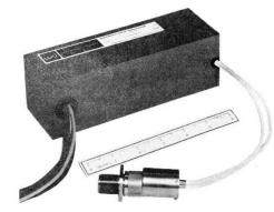
Cathode modulation with the grid grounded usually reduces FM caused by AM. With all voltages isolated from both tube housing and the r.f. output terminal, packaging problems are simplified, since the tube housing and output connector can be grounded regardless of power supply configuration.
