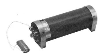
operation. It may be operated in any orientation. Rugged construction of the tube, magnet, and power supply assembly ensures reliable operation under vibrational forces of 10 g, at frequencies up to 500 Hz. Full specifications are met over the operating temperature range of -54 °C to +71 °C. The environmental characteristics of the WJ-460 meet or exceed the corresponding requirements of MIL-E-5400, class 2 specification.
