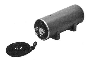
WJ-3003 is an S-band amplifier that provides 100 mW power output for applications where increased dynamic range is desired. The amplifier is completely self-contained, adjustment-free, and requires only a 115-volt ac line voltage input (48 to 420 Hz). In addition, it may be operated in any orientation, in stacked arrays, or adjacent to ferromagnetic materials without degradation of performance.
