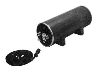
WJ-3005 is an X-band amplifier that provides 100 mW power output for applications where increased dynamic range is desired. The amplifier is completely self-contained, adjustment-free, and requires only a 115-volt ac line voltage input (48 to 420 Hz). In addition, it may be operated in any orientation, in stacked arrays, or adjacent to ferromagnetic materials without degradation of performance.
