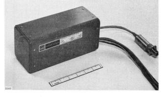
low operating cathode current. Power can be modulated and leveled with either grid or anode circuit. All voltages are isolated from housing and RF output connector for maximum flexibility in circuit applications.
