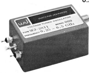
WJ-2811 is a voltage-tuned transistor oscillator designed to provide fundamental microwave power over the 0.25 to 0.5 GHz range. Varactor tuning ensures a high tuning input impedance characteristic for the device. Since it is a fundamental oscillator, no inband harmonics are exhibited.
