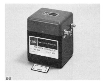
A special feature of the WJ-700 is its compatibility with the WJ-723 three-stage YIG filter. The resulting harmonic generator filter chain provides microwave harmonic energy with over 100 dB suppression of harmonics spaced  $\pm 200$  MHz or more from the tuned harmonic when driven by less than one watt of 100 MHz fundamental signal.
