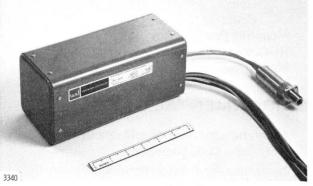
grain variation of frequency versus voltage is extremely low. Power output and tuning curves are uniform and highly reproducible. Power can be modulated and leveled with either grid or anode circuits. All voltages are isolated from housing and RF output connector for maximum flexibility in circuit applications.
