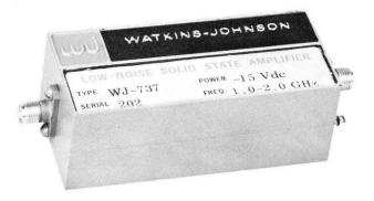
Modular construction ensures high reliability under adverse operating conditions. Calculated MTBF for this amplifier exceeds 225,000 hours. The microstripline circuit configuration employs integrated circuit biasing and bypass modules for consistently high performance. The overall design of the WJ-737 is consistent with the general requirements of MIL-E-16400 and MIL-E-5400, class II. Since the amplifier is tested and set for operation prior to shipment, no adjustments are necessary by the user.
