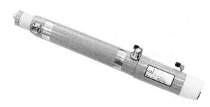
The WJ-228 is a high-power, high-gain C-band traveling-wave amplifier for pulsed operation. This tube is of rugged, light-weight construction backed by production experience gained through the manufacture of large quantities of this type. The WJ-228 produces 14 kw power output with 0.5 watt drive. It employs a high-mu grid which permits modulation of the beam by means of a 50C-volt pulse.
