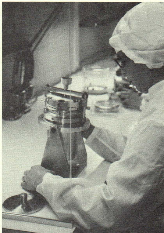
The screened bulb and the mesh are assembled at a clean horizontal-flow bench with unique fixtures used to accomplish the required precision.
