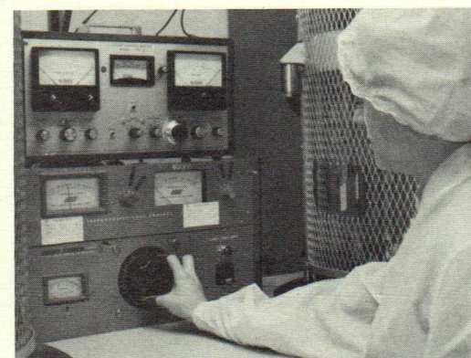
Careful monitoring of dielectric parameters assure continuous control in display storage tube production.
