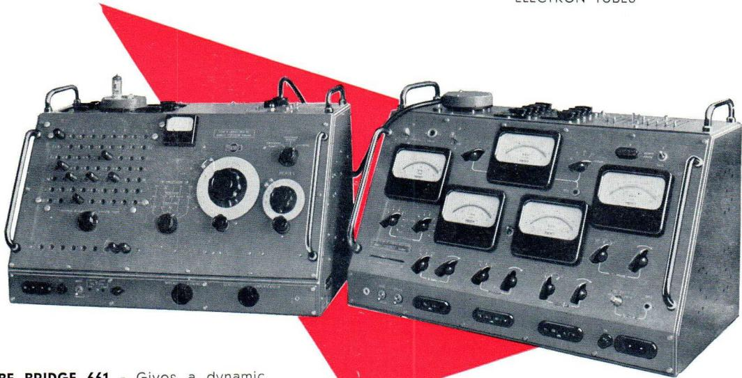
**VACUUM TUBE BRIDGE 661** - Gives a dynamic measurement of internal resistance, mutual conductance, and amplification factor at any point on the static characteristics. DC and heater power for the tube under test may be supplied by the U 61 B.
