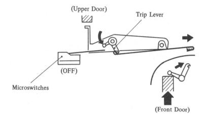
Fig. 4-117 Door Switch Group Operation (B)
