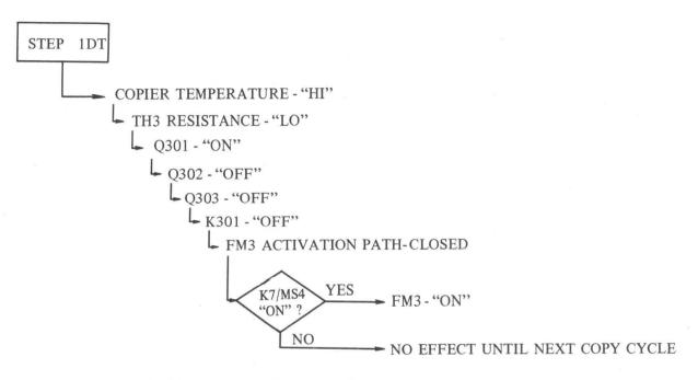
Fig. 3-15 Developer Cooling Flowchart
