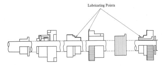
Fig. 4-85 Timing roller Drive Lubrication
