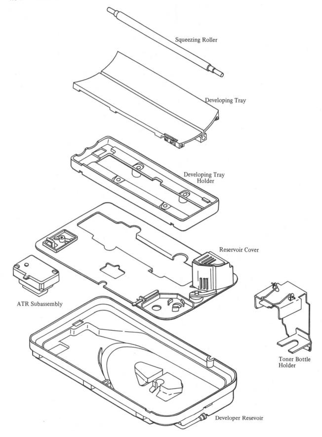
Fig. 4-35 Developer Assembly Main Components
