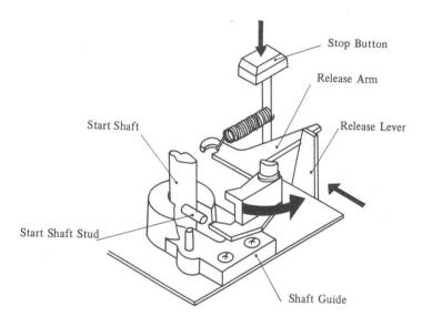
Fig. 4-110 Stop Button Operation
