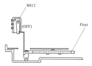
Fig. 4-45 Normal Developer Level
