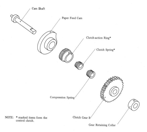
Fig. 4-75 Paper Feed Cam Drive Main Components
