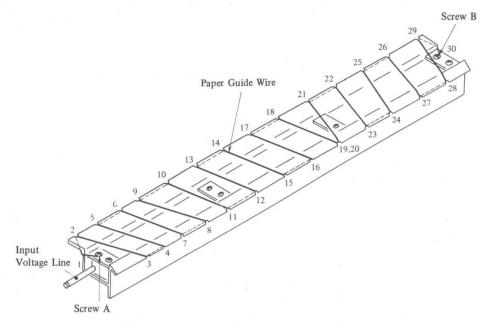
Fig. 4-30 Paper Guide Wire Replacement of Residual Charge Eliminator Assembly
