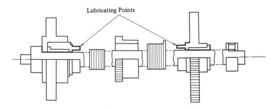
Fig. 4-84 Paper Feed Cam Drive Lubrication
