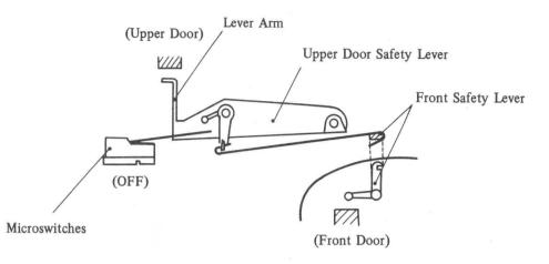
Fig. 4-116 Door Switch Group Operation (A)
