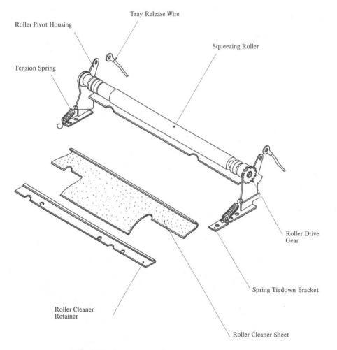
Fig. 4-40 Squeezing roller Main Components
