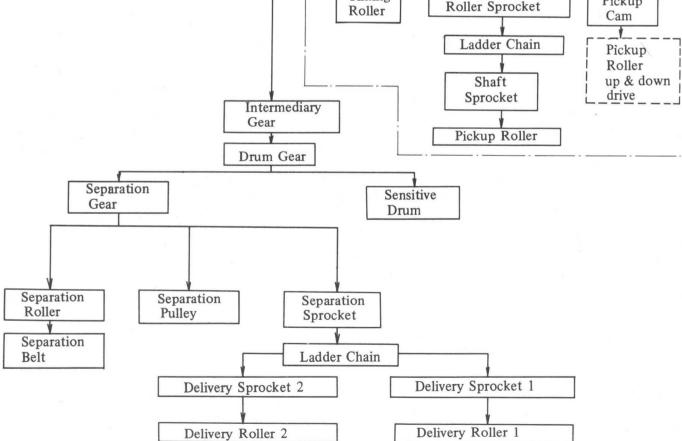
Fig. 2-5 Block Diagram of the Drive System
