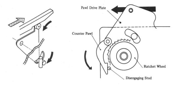
Fig. 4-108 Copy Selector Operation (C)
