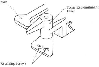
Fig. 4-49 Replenishment Lever Adjustment
