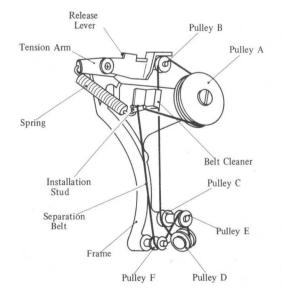
Fig. 4-97 Paper Separating Subassembly Main Components
