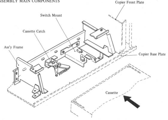
Fig. 4-56 Cassette Holder Assembly Main Components
