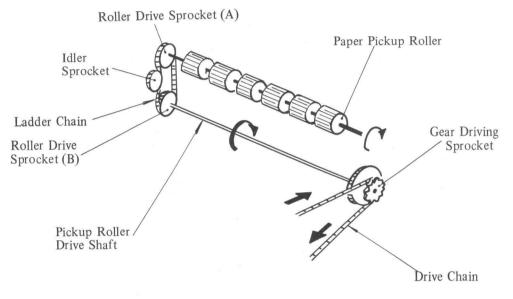
Fig. 4-58 Pickup Roller Rotation Drive
