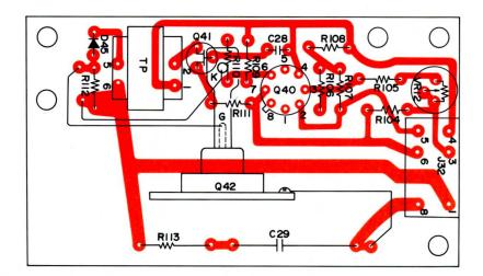
Heater Control Circuit - 100VAC Only (P. C. Assembly 5)
