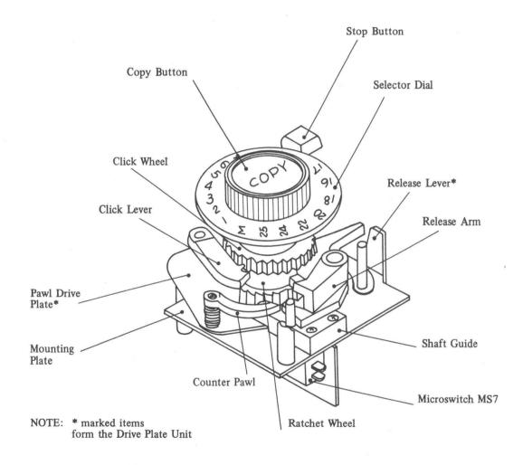
Fig. 4-104 Copy Selector Subassembly Main Components
