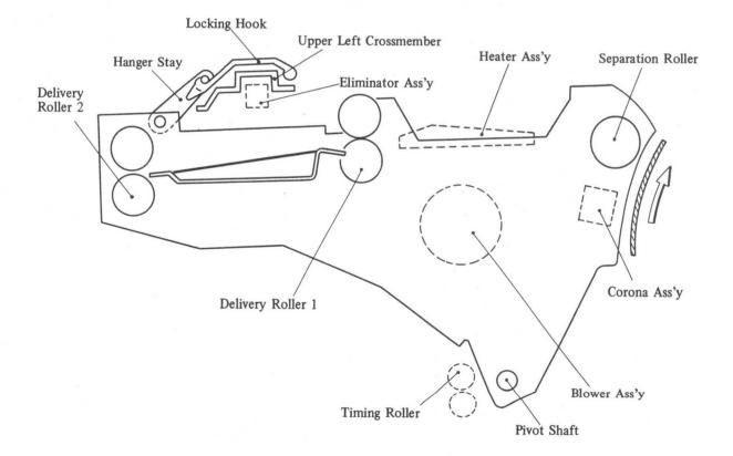
Fig. 4-90 Copy Conveying Assembly (from copier front)
