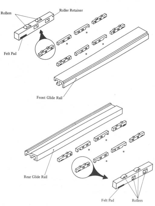
Fig. 4-4 Roller Unit Positioning
