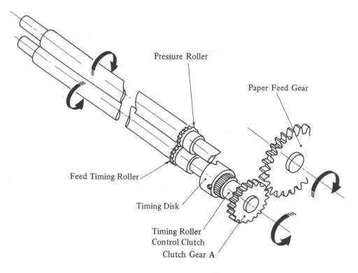
Fig. 4-61 Timing Roller Drive Components
