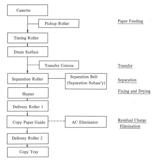
Fig. 2-9 Diagram of Copy Paper Movement
