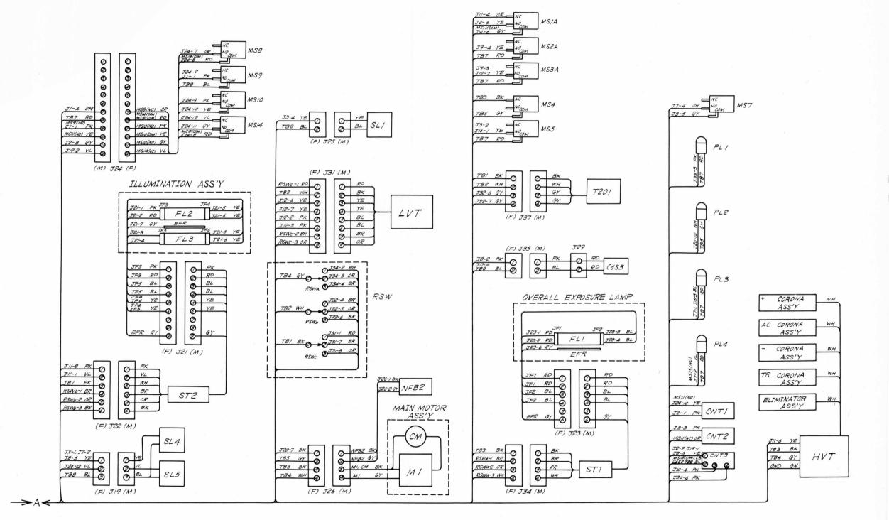
Photocopier Wiring Diagram, Prod. No. 8-11154/55 (2 of 2)
