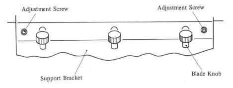
Fig. 4-55 Adjustment of Cleaner Blade Pressure (B)
