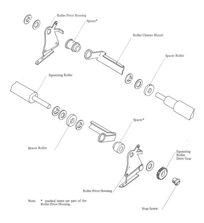
Fig. 4-48 Components of Squeezing Roller (Detailed)
