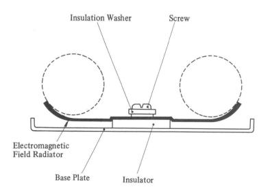
Fig. 4-15 Electromagnetic Field Radiator Mounting
