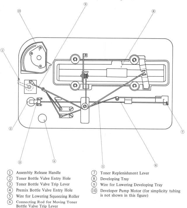
Fig. 4-41 Reservoir Cover Components (Underside View)
