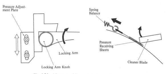
Fig. 4-54 Adjustment of Cleaner Blade Pressure (A)
