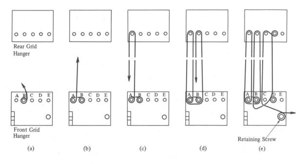
Fig. 4-33 Wiring Procedure
