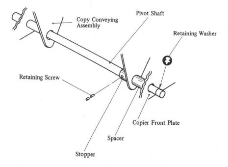
Fig. 4-91 Pivot Shaft Removal
