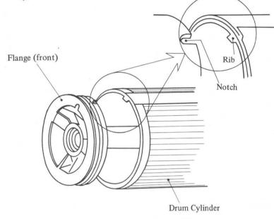
Fig. 4-28 Drum Unit Reassembly
