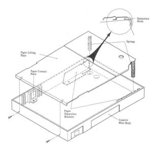
Fig. 4-57 Cassette Assembly Main Components
