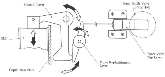
Fig. 4-43 Replenishing Mechanism Main Components
