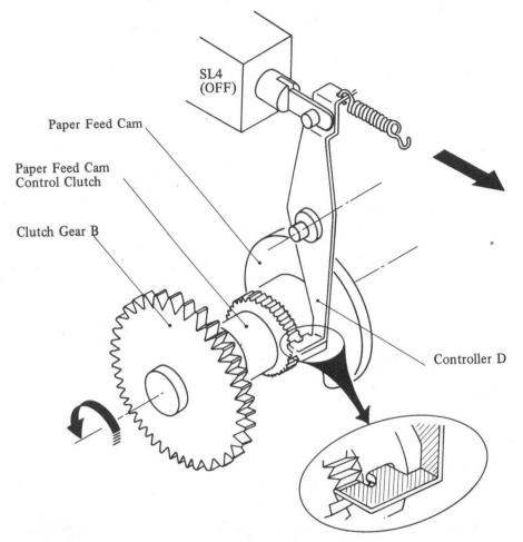
Fig. 4-62 Controller Assembly Operation (A)
