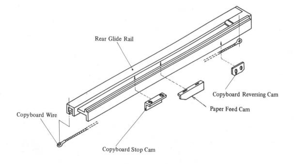
Fig. 4-3 Rear Rail Components
