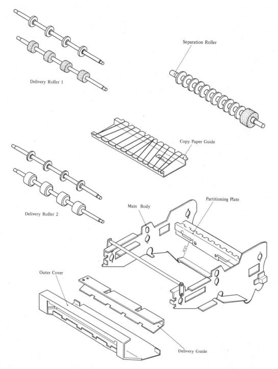
Fig. 4-86 Copy Conveying Assembly Main Components
