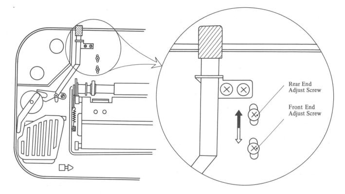
Fig. 4-50 Squeezing Roller Adjustment
