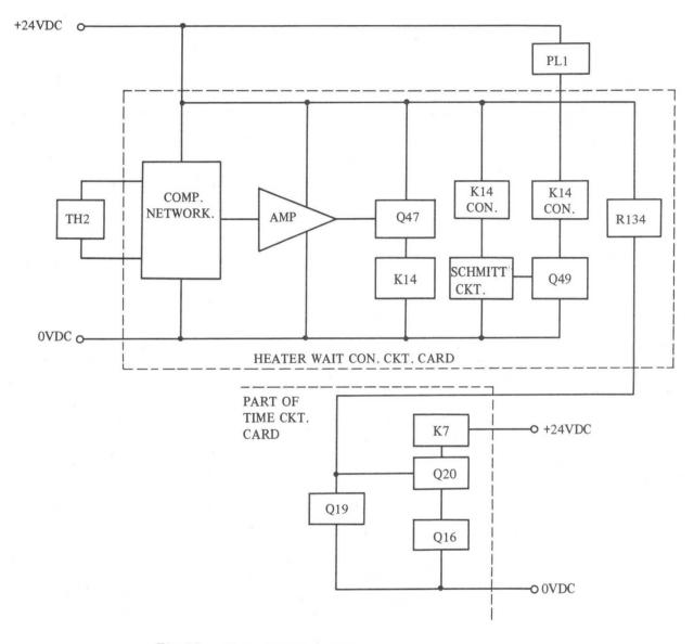
Fig. 3-9 Heater Wait Control Circuit & Associated Components
