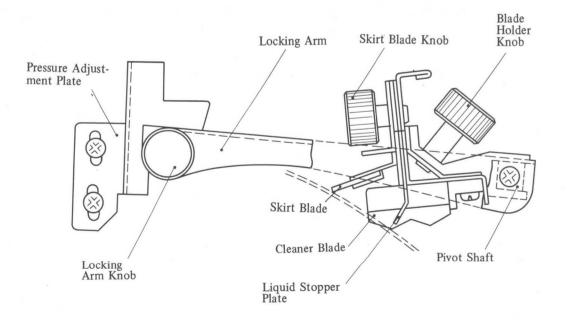
Fig. 4-52 Drum Cleaner Assembly Main Components (from Copier Front)
