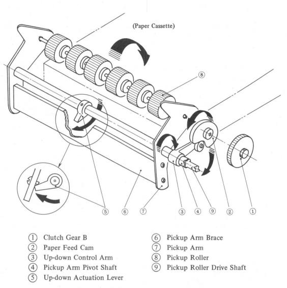
Fig. 4-59 Roller Up-down Drive Components
