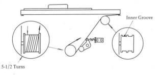
Fig. 4-6 Copyboard Wire Installation (B)
