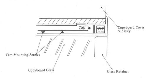
Fig. 4-11 Location of Paper Feed Cam
