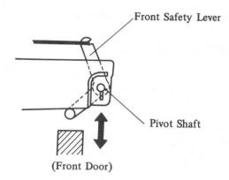
Fig. 4-123 Adjustment of Front Safety Lever
