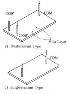
Fig. 4-99 Heater Element Types
