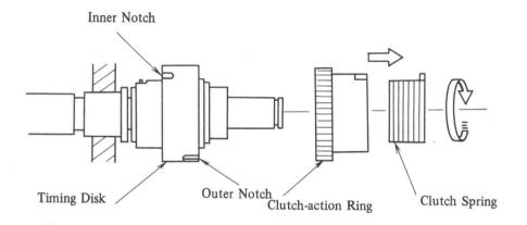
Fig. 4-74 Timing Roller Drive Disassembly (B)
