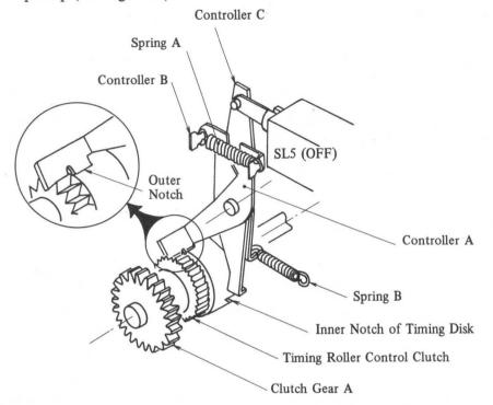
Fig. 4-66 Controller Assembly Operation (E)
