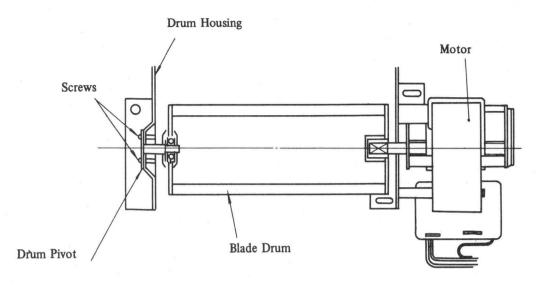
Fig. 4-103 Blower Blade Drum Adjustment
