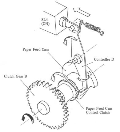
Fig. 4-64 Controller Assembly Operation (C)
