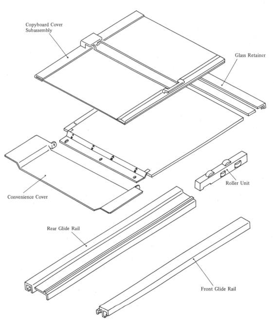
Fig. 4-1 Copyboard Assembly Main Components
