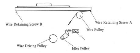
Fig. 4-5 Copyboard Wire Installation (A)
