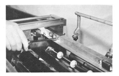
Fig. 4-29 Eliminator Assembly Removal
