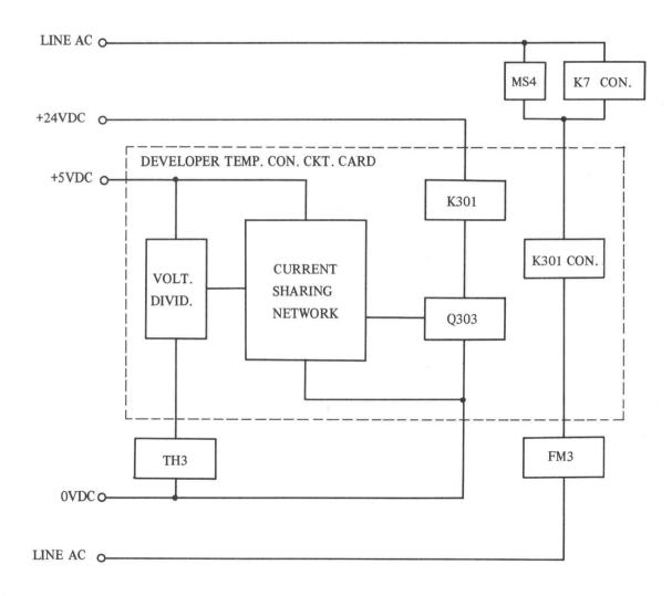
Fig. 3-14 Developer Temperature Control Circuit & Associated Components
