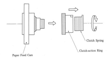
Fig. 4-78 Paper Feed Cam Drive Disassembly (C)
