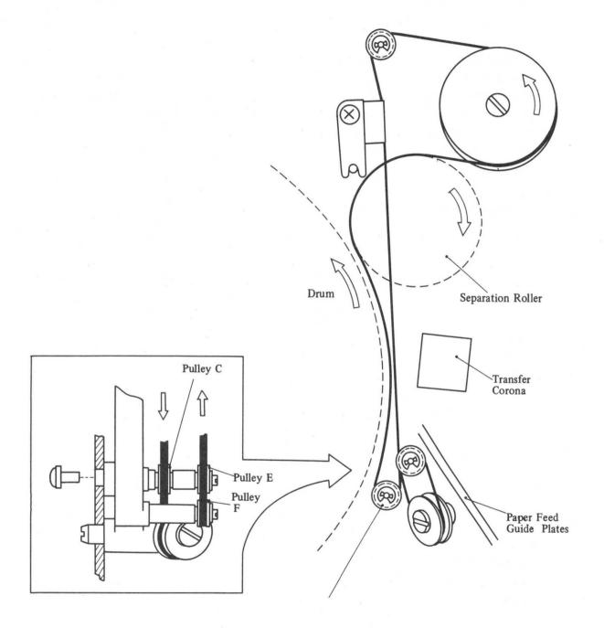
Fig. 4-96 Movement of Separation Belt (from copier rear) Fig. 4-96 depicts the Paper Separating Subassembly in its normal operating position. As the main drive motor (M1) turns the drum, the separation roller is also driven (see arrows). The movements of these components drive the separation belt around its endless path at the same rate of speed as the drum.
