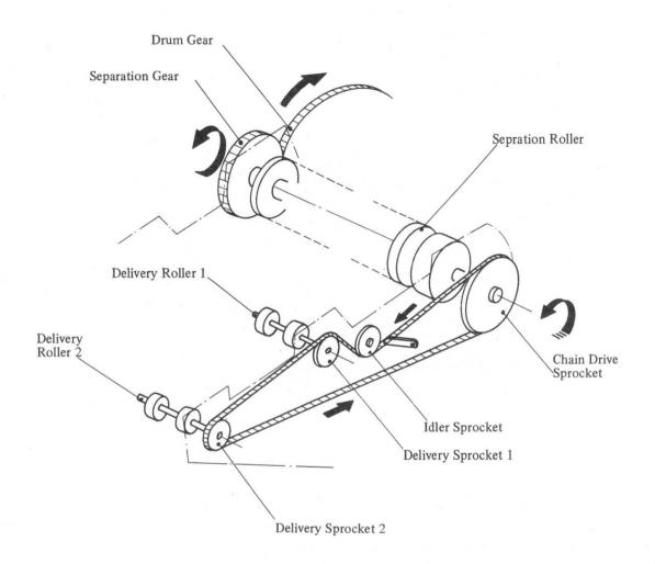
Fig. 2-8 Conveying Drive Mechanism
