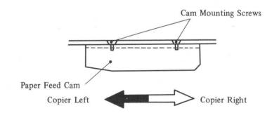
Fig. 4-12 Paper Feed Cam Adjustment
