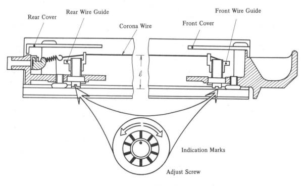
Fig. 4-34 Corona Wire Adjustment (Positive Corona Assembly illustrated)
