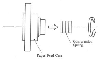
Fig. 4-79 Paper Feed Cam Drive Disassembly (D)
