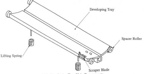
Fig. 4-39 Developing Tray Main Components
