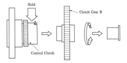
Fig. 4-77 Paper Feed Cam Drive Disassembly (B)
