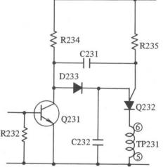
Fig. 3-24 1/1 Zero-Cross Circuit
