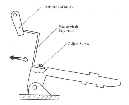
Fig. 4-51 Developer Float Adjustment
