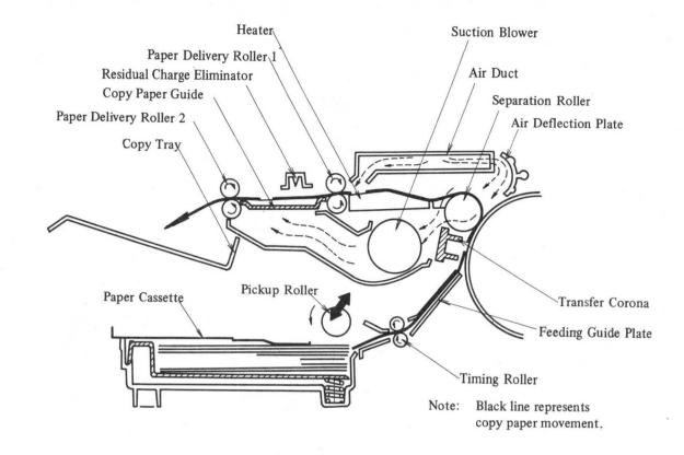
During the copying process, copy paper moves through the machine in the manner shown below.
