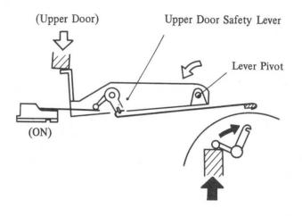
Fig. 4-118 Door Switch Group Operation (C)
