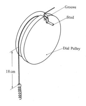
Fig. 4-20 Adjust Line Replacement (A)
