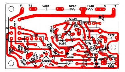
Heater Control Circuit - "Zero-Cross" (P. C. Assembly 5)
