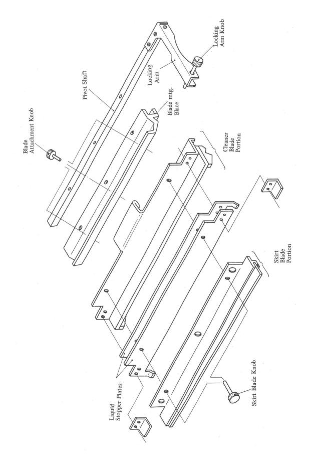
Fig. 4-53 Drum Cleaner Assembly Main Components (Exploded View)
