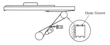
Fig. 4-7 Copyboard Wire Installation (C)
