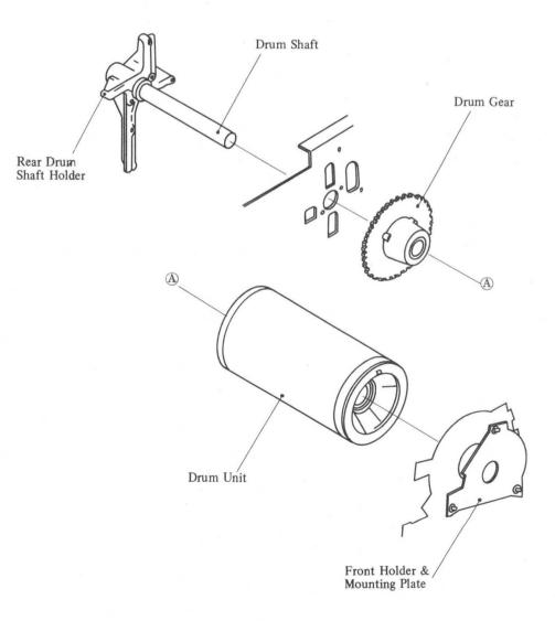
Fig. 4-25 Drum Assembly Main Components
