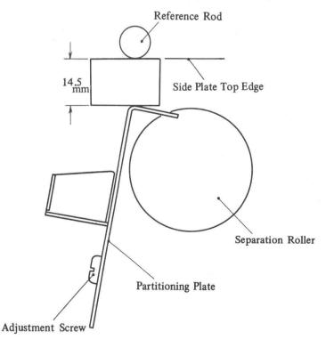
Fig. 4-94 Partitioning Plate Height Adjustment
