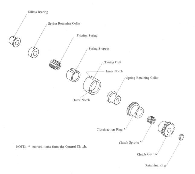
Fig. 4-72 Timing roller Drive Main Components
