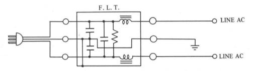
Fig. 3-5 Low-Pass Filter-Schematic Diagram
