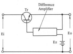
Fig. 3-6 Voltage Regulator – Typical
