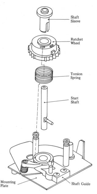
Fig. 4-112 Copy Selector Reassembly
