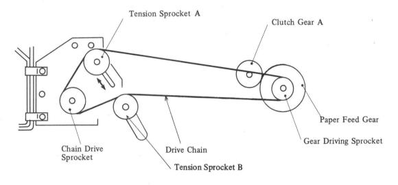
Fig. 4-71 Drive Chain Removal
