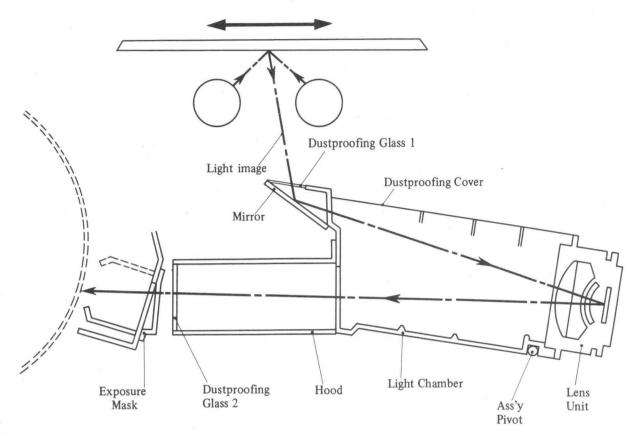
Fig. 4-18 Optical Assembly Main Components
