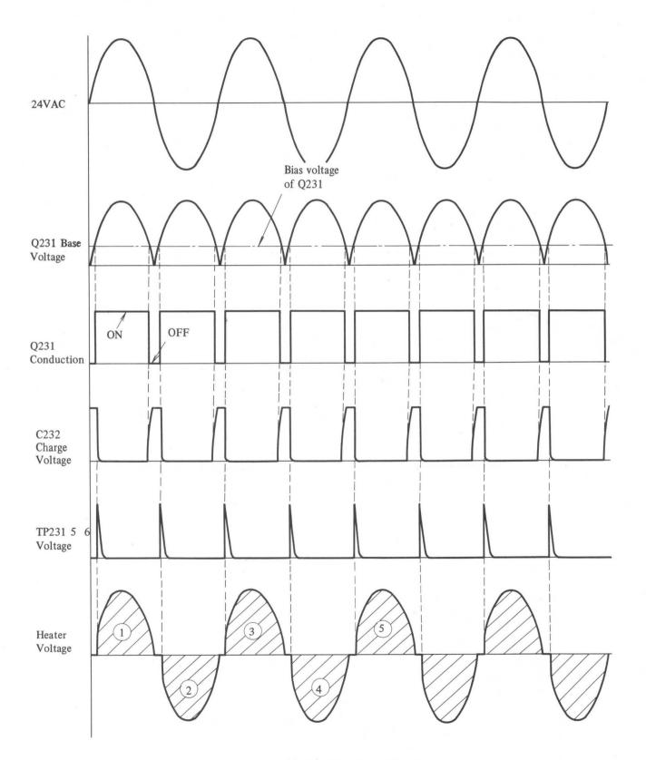
Fig. 3-25 depicts the waveforms for the operation of the 1/4 zero-cross circuit.
