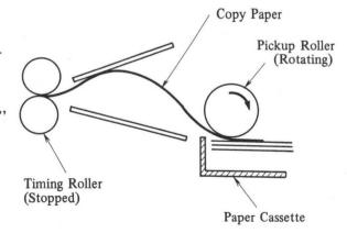
Fig. 4-67 Controller Assembly Operation (F)
