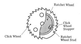
Fig. 4-113 Click and Ratchet Wheel Positioning (Top View)
