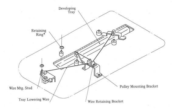
Fig. 4-47 Reservoir Cover (Underside View)
