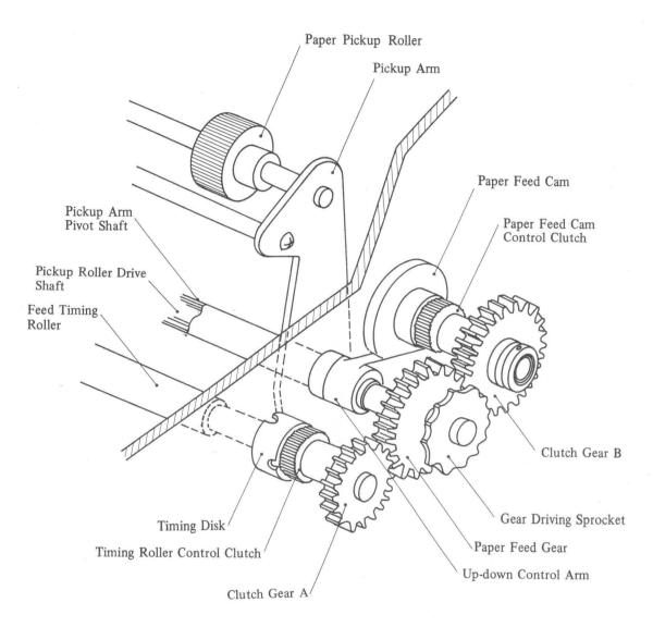
Fig. 4-70 Paper Pickup Roller Assembly Main Components
