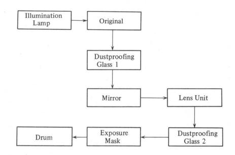
Fig. 4-17 Block Diagram of Light Travel
