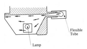
Fig. 4-37 Developer Flow Through ATR Subassembly
