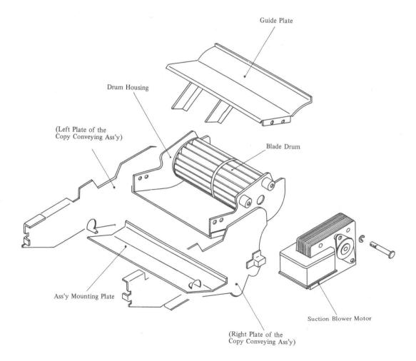
Fig. 4-100 Suction Blower Assembly Main Components
