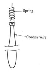
Fig. 4-32 Attaching Corona Wire
