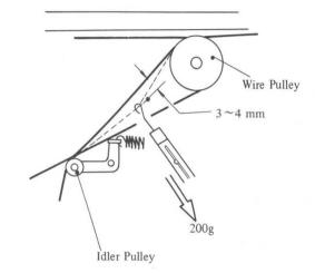
Fig. 4-9 Measuring of Wire Tension
