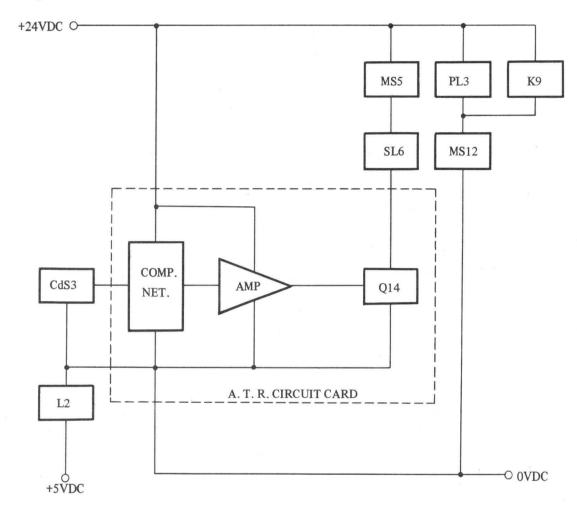
Fig. 3-11 Developer Monitoring Circuitry
