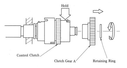
Fig. 4-73 Timing Roller Drive Disassembly (A)
