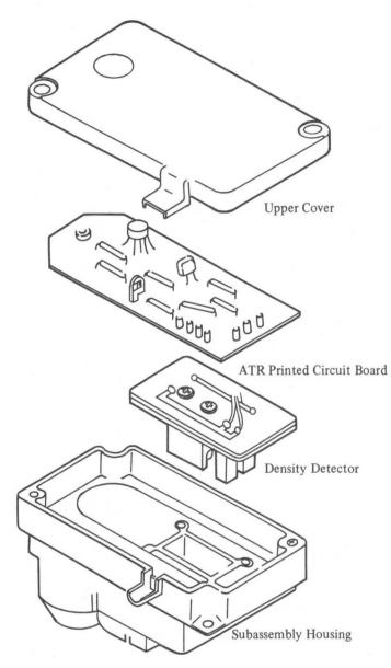
Fig. 4-36 ATR Subassembly Main Components
