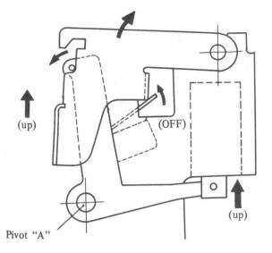
Fig. 4-122 Jam Stop Group Operation (B)
