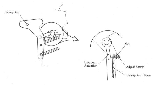
Fig. 4-83 Pickup Roller Height Adjustment
