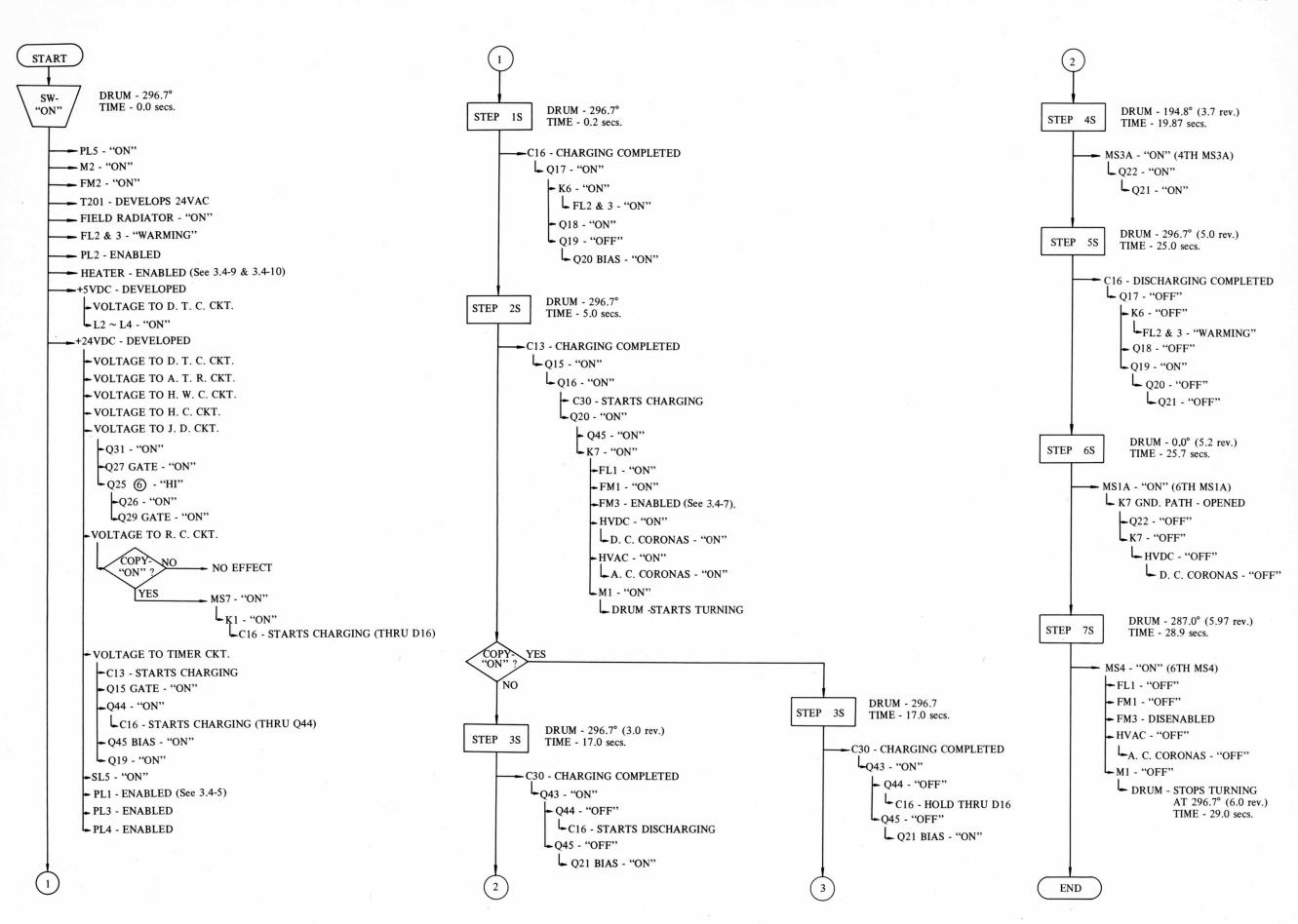
Fig. 3-1 (START) Flowchart (Sheet 1 of 1)
