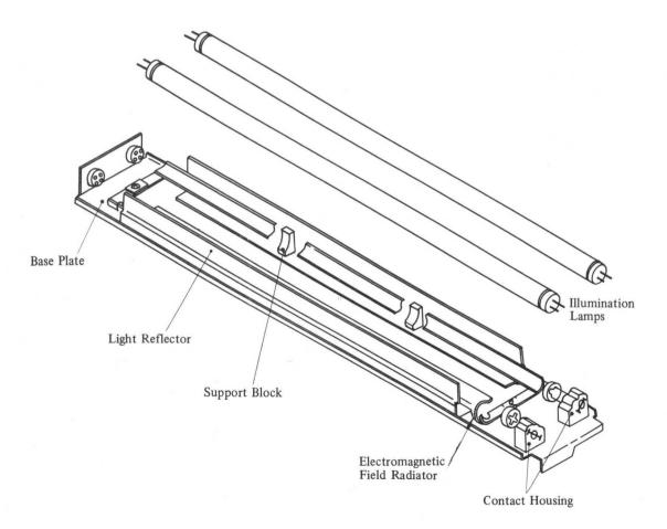
Fig. 4-13 Illumination Assembly Main Components
