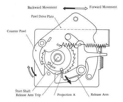
Fig. 4-109 Copy Selector Operation (D)
