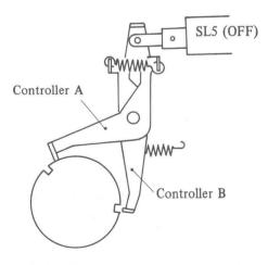
Fig. 4-65 Controller Assembly Operation (D) vi) The timing roller stops when controller A falls into the outer notch of the timing disk and, thus, engages the timing roller control clutch. During this time, however, the paper feed control cam is still operating the up-down control arm to cause paper pickup (see Fig. 4-66).
