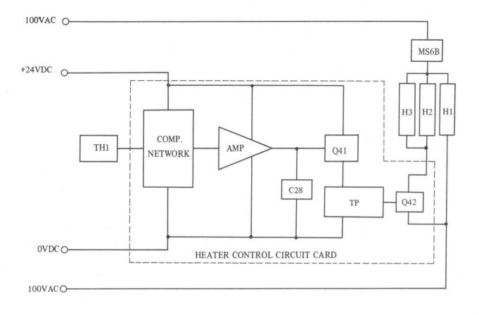
Fig. 3-19 Heater Control Circuit & Associated Components
