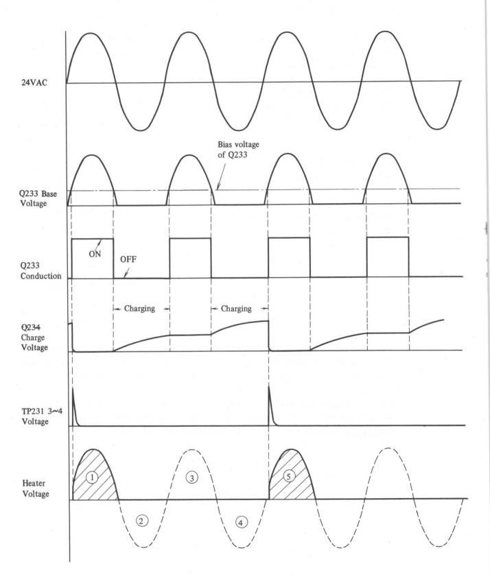
Fig. 3-23 depicts the waveforms for the operation of the 1/4 zero-cross circuit.
