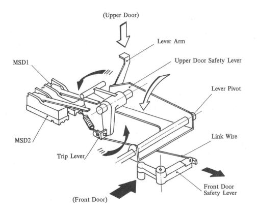
Fig. 4-115 Door Switch Group Main Components
