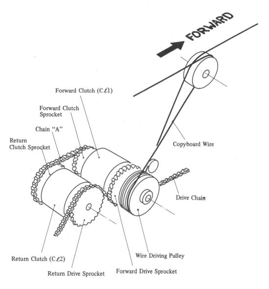
Fig. 4-129 Copyboard Driving Mechanism Assembly Main Components
