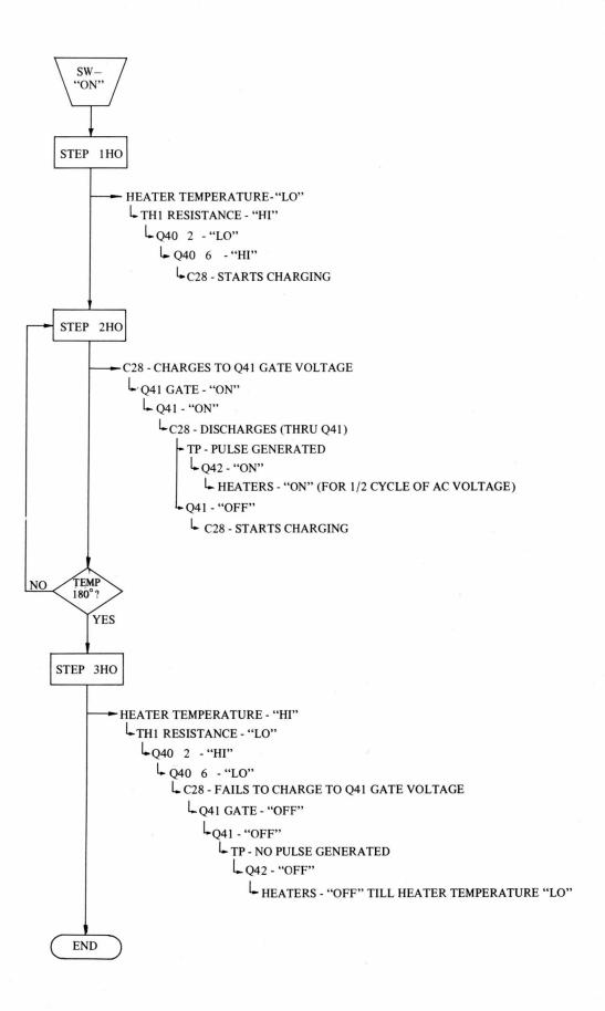
Fig. 3-20 Heater Operation Flowchart
