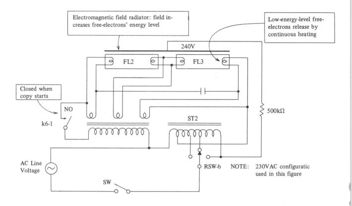
Fig. 3-8 Original Illumination Circuit
