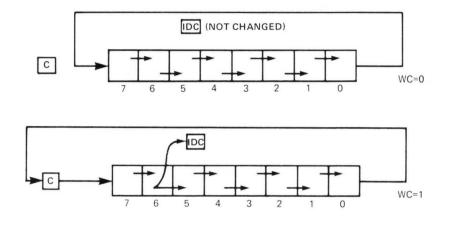
**Note:** Whenever a rotate causes bit #7 of the specified register to change polarity, the OVF bit is set in the PSL.
