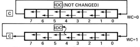
**Note:** Whenever a rotate causes bit #7 of the specified register to change polarity, the OVF bit is set in the PSL.
