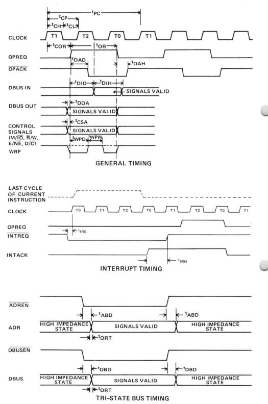
Figure 9. 2650 TIMING DIAGRAMS
