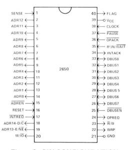
Figure 3. PIN CONFIGURATION
