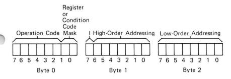
The notable difference is that bits 6 and 5, byte 1, are no longer interpreted as Index Control bits, but instead are interpreted as the high order bits of the address field. This means that there is no indexing allowed on most absolute addressing branch instructions, but indexed branches are possible through use of the BXA and BSXA instructions. The bits #6 and #5, byte 1, are used to set the current page register, thus enabling programs to directly transfer control to another page.
