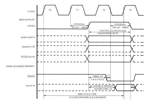
NOTES: (1) OPACK must go low at least 100 nS before the trailing edge of T2 in order not to slow down the 2650. (2) DATA IN signals must be valid for 50nS after the trailing edge of OPREQ. (3) Allowable memory access time is 1µs with 2.4µs cycle time.
