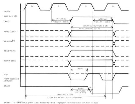
Figure 11 demonstrates the signals that occur during a memory write.
