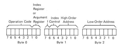
Bits 4-0, byte 1 and 7-0, byte 2 contain the absolute address and can address any byte within the same page that the instruction appears.
