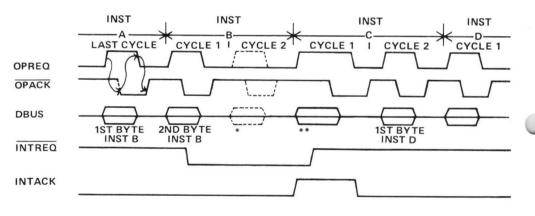
PROCESSOR INSERTS 1ST BYTE OF ZBSR INSTRUCTION. ADDRESS OF 1ST BYTE OF INSTC IS PUSHED INTO RETURN ADDRESS STACK.
