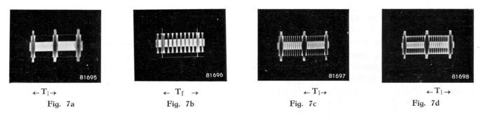
Oscillograms of the H.F. output voltage a) Blank field, b) horizontal bars, c) vertical bars, d) horizontal and vertical bars  $T_1 =$  line period,  $T_f =$  field period
