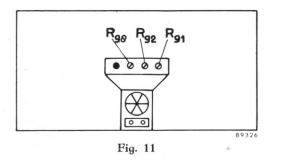
must function properly. The correct number of blocks in vertical direction (6) can be adjusted. by  $R_{91}$ , while  $R_{92}$  is provided for adjustment of the correct number (8) in horizontal direction. Furthermore it is possible to equalize the width of the black interstices between the blocks in horizontal and vertical direction by means of  $R_{98}$ .
