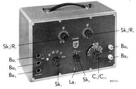
Fig. 17. Nomenclature of knobs and sockets
