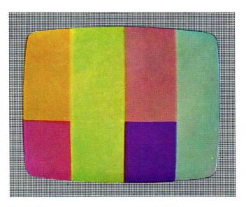
Fig. VII-21. Incorrect subcarrier phase to the (B-Y) demodulator
