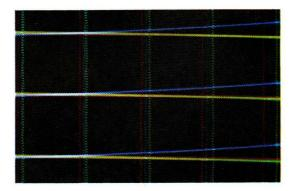
Fig. VII-12. Picture detail in case of incorrect dynamic convergence
