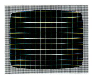
Fig. VII-11. Incorrect horizontal dynamic convergence
