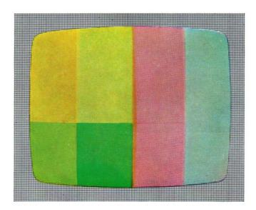
Fig. VII-20. Incorrect subcarrier phase to the (R-Y) demodulator
