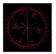
Fig. VII-24. Vectorscope display of the "MATRIX"-pattern
