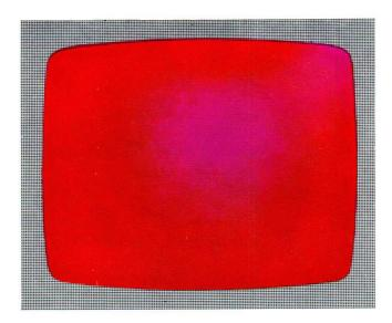
Fig. VII-6. Typical purity error
