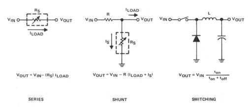
Figure 1.2. Control Element Configurations
