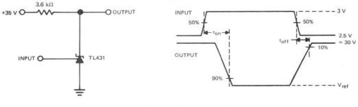
FIGURE 3-TEST CIRCUIT FOR ton AND toff
