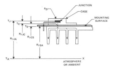
Figure 5.1. Semiconductor Thermal Model
