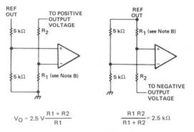
FIGURE 6-ERROR AMPLIFIER BIAS CIRCUITS
