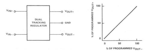
Figure 3.4. Dual Tracking Regulator
