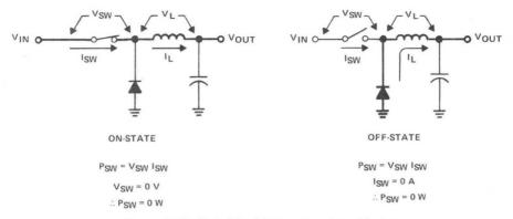
Figure 3.10. Switching Voltage Regulator Modes
