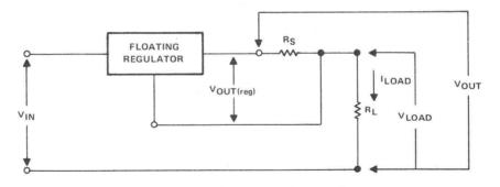
Figure 3.7. Floating Regulator as a Constant-Current Regulator
