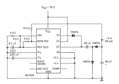
FIGURE 12-CAPACITOR-DIODE OUTPUT CIRCUIT
