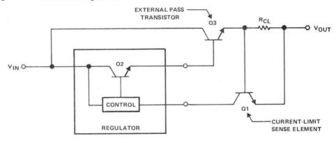
Figure 4.6. Constant-Current Limiting for External Pass Transistor Applications
