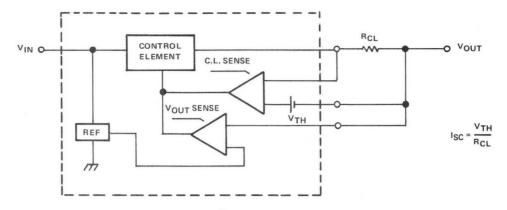
Figure 4.5. Constant Current Limit Configuration
