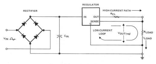
Figure 6.2. Proper Regulator Layout
