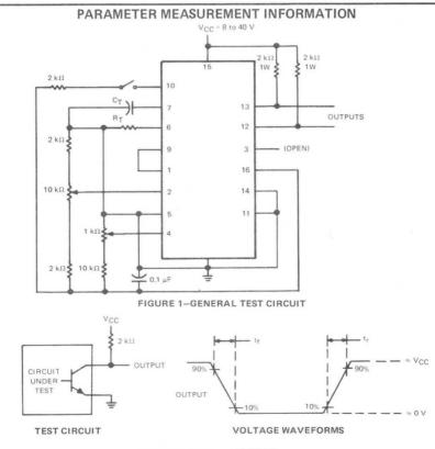
FIGURE 2-SWITCHING TIMES
