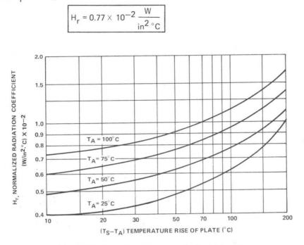
Figure 5.7. Normalized Heat Transfer Coefficient H<sub>r</sub>
