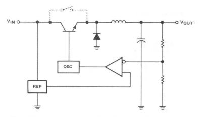
Figure 1.5. Basic Switching Regulator (Step-Down Configuration)
