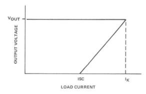
Figure 4.8. Fold-Back Current Limiting
