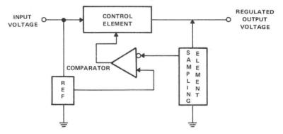
Figure 1.1. Basic Regulator Block Diagram
