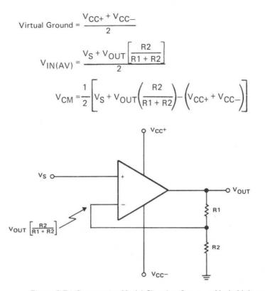
Figure 2.7. Comparator Model Showing Common-Mode Voltage
