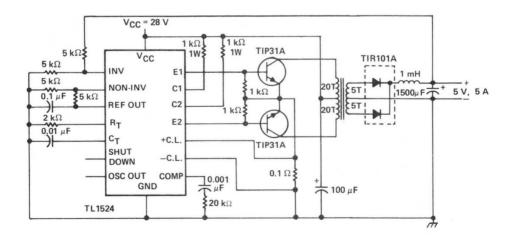
FIGURE 15-PUSH-PULL TRANSFORMER-COUPLED CIRCUIT
