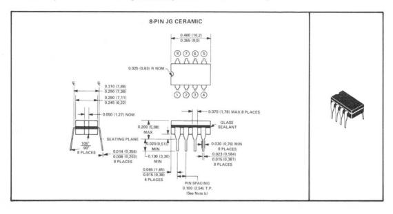
NOTES: a. All dimensions are in inches and parenthetically in millimeters. Inch dimensions govern. b. Each pin centerline is located within 0.010 (0,26) of its true longitudinal position.
