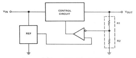
Figure 2.5. R1/R2 Ladder Network Sampling Element
