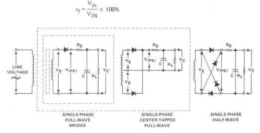
Figure 7.8. Input Filter Design
