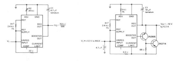
FIGURE 1-BASIC REGULATOR CIRCUIT
