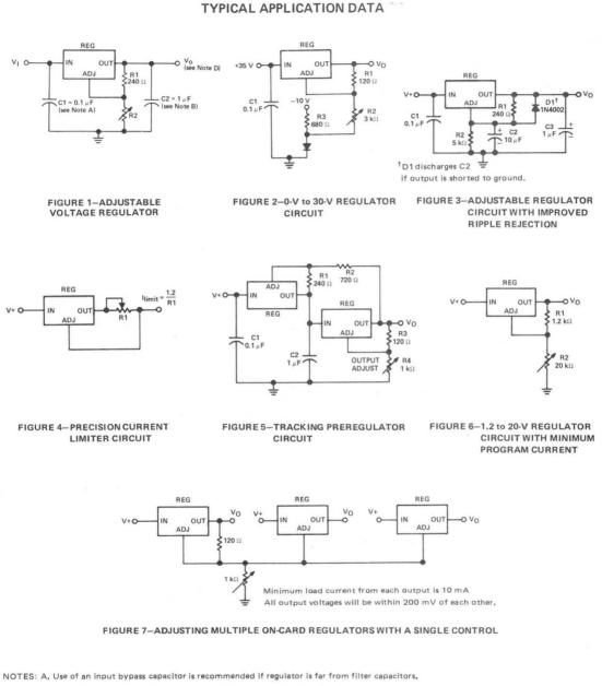
B. Use of an output capacitor improves transient response but is optional.
