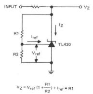
FIGURE 1-TEST CIRCUIT FOR VZ = Vref
