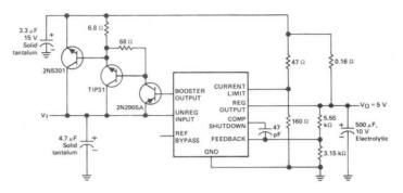
FIGURE 3-10-A REGULATOR WITH FOLDBACK CURRENT LIMITING
