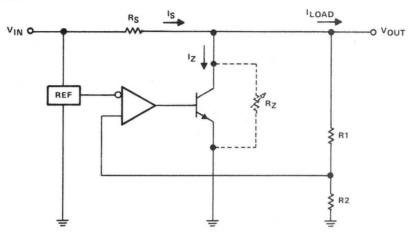
Figure 1.4. Basic Shunt Regulator
