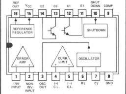
The SG1524 is characterized for operation over the full military temperature range of  $-55^{\circ}$ C to  $125^{\circ}$ C. The SG2524 and SG3524 are characterized for operation from 0°C to 70°C.
