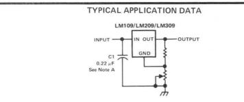
NOTE A: C1 is required if regulator is not located in close proximity to power supply filter.
