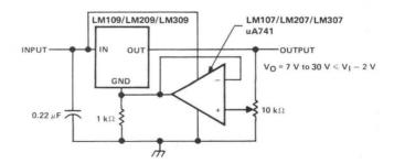
FIGURE 13-HIGH-STABILITY REGULATOR WITH ADJUSTABLE OUTPUT
