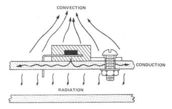
Figure 5.3. Heat Flow Paths of Semiconductor Cooling
