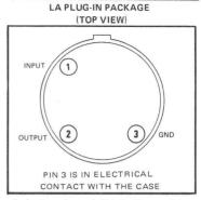
These monolithic 5-volt regulators are designed for use as local regulators to eliminate noise and distribution problems inherent with single-point regulation. They are specified under worst-case conditions to match the power supply requirements of TTL and DTL logic families. In other applications, these devices can be used with external components to obtain adjustable output voltages and currents or as the series-pass element in precision regulators.
