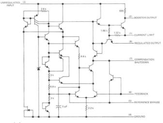
Component values shown are nominal. Resistor values are in ohms.
