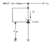
FIGURE 1-TEST CIRCUIT FOR VZ = Vref
