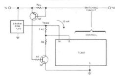
DESIGN EQUATIONS  $R_{CL} = \frac{V_{BE(Q1)}}{I_{LIMIT(PK)}}$   $R1 = \frac{V_{I}}{I_{B(Q2)}}$   $R2 = (V_{REG} - 1) \ 10 \ k\Omega$
