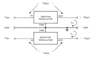
Figure 3.1. Conventional Positive/Negative Regulator
