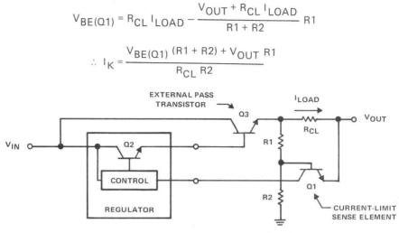
Figure 4.9. Fold-Back Current Limit Configuration
