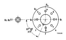
Mounting position: any, except vertical with the screen down and the axis of the tube making an angle of less than  $20^{\circ}$  with the vertical.
