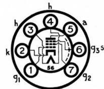
The BRIMAR 6064 is an indirectly-heated high slope R.F. Pentode suitable for a wide variety of applications. It may be used as an R.F. or I.F. or video amplifier, as a limiter, or as a frequency changer at frequencies up to 100 Mc/s in conjunction with a suitable oscillator.
