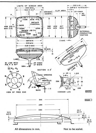
It is recommended that the mask used with this tube is flexible enough to take up small variations in fixing and bulb contours.
