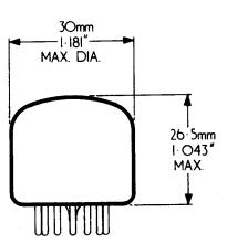
The dome of the tube is filter coated
