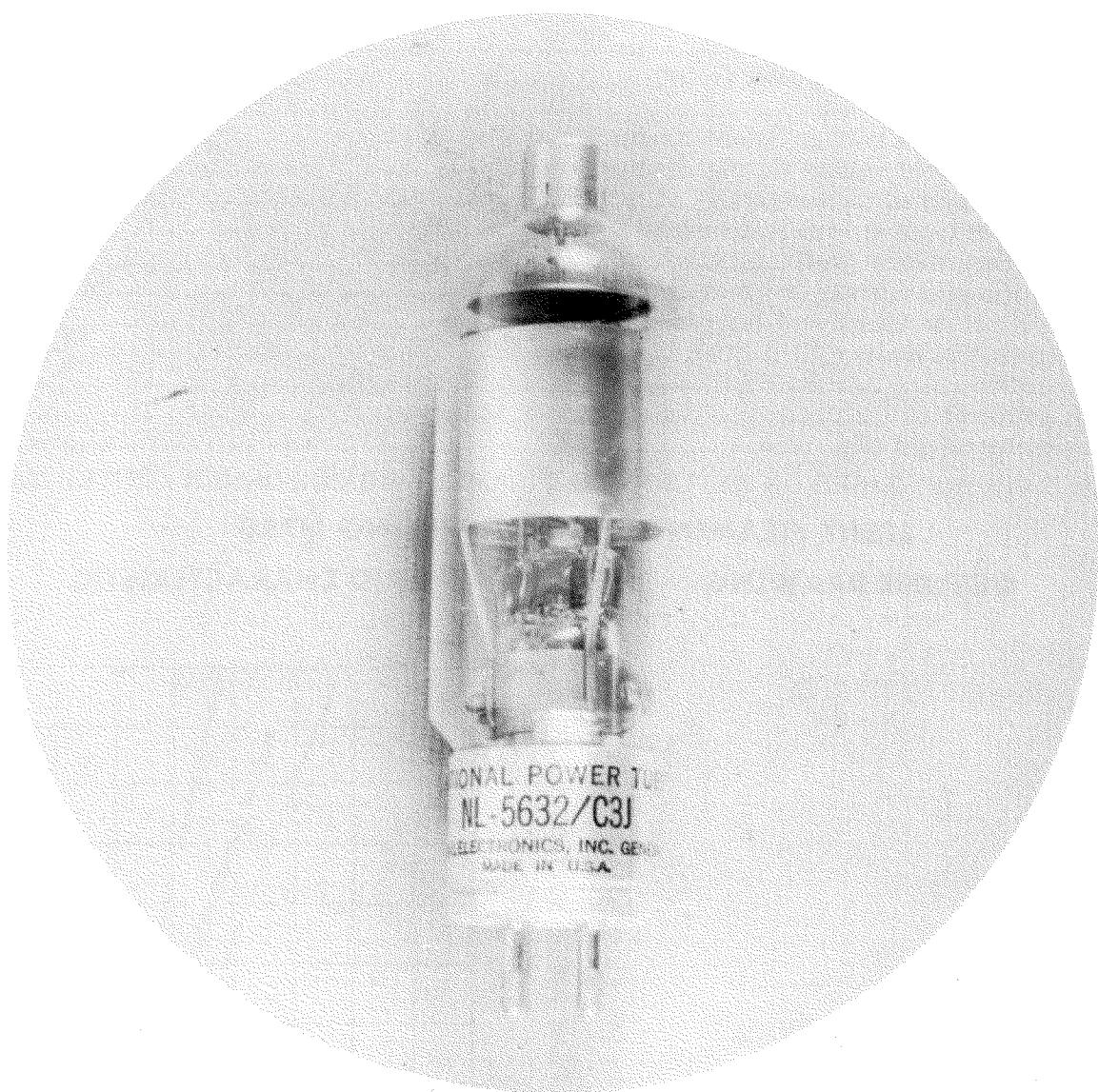
NATIONAL POWER TUBE NL-5632/C3J is a quick heating thyratron designed for timing and control applications. It is xenon filled for quick starting and the ability to operate within wide ambient temperature limits. It is ruggedly constructed for industrial applications.
