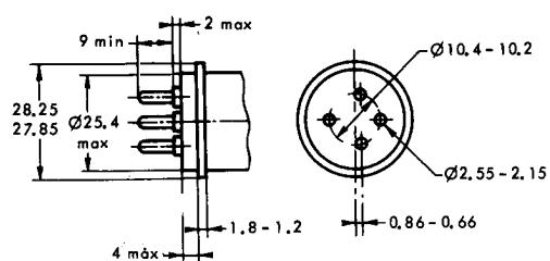
The pin position with respect to the tube axes is determined within 10°
