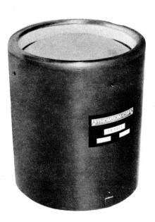
TH 9427 is delivered in a shell which permits mechanical mounting, protects the tube from stray magnetic field and secures a precise positioning of the associated optical system.
