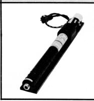
The EM-1050 features rugged ceramic and metal construction and focusing is provided by built-in periodic permanent magnets. These magnets are fully temperature compensated to allow operation from -55 to  $+85^{\circ}$ C. No additional cooling is required at these temperatures due to the integral heat sink/mounting flange supplied with the tube.
