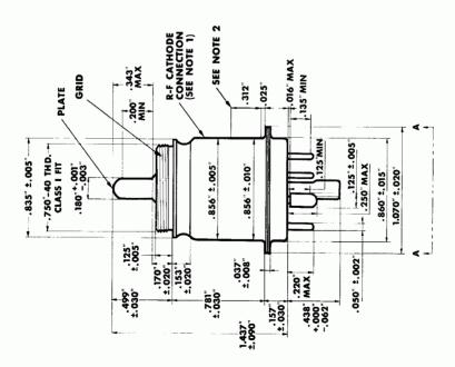
NOTE 1: Surfaces of R-F cathode, grid, anode and pin connections are gold plated. NOTE 2: .856" $\pm$  .010" dimension applies only over the .312" length.
