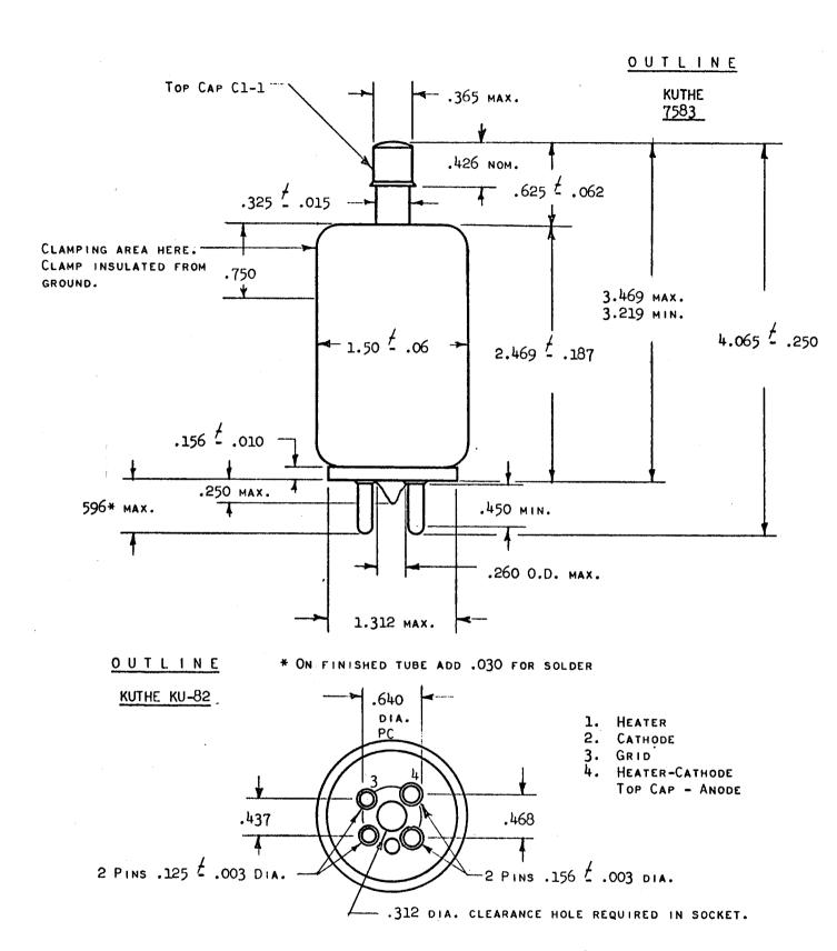
WAFER BASE. PIN ARRANGEMENT AND DIMENSIONS ONLY AS PER A4-9 MIL-E-10
