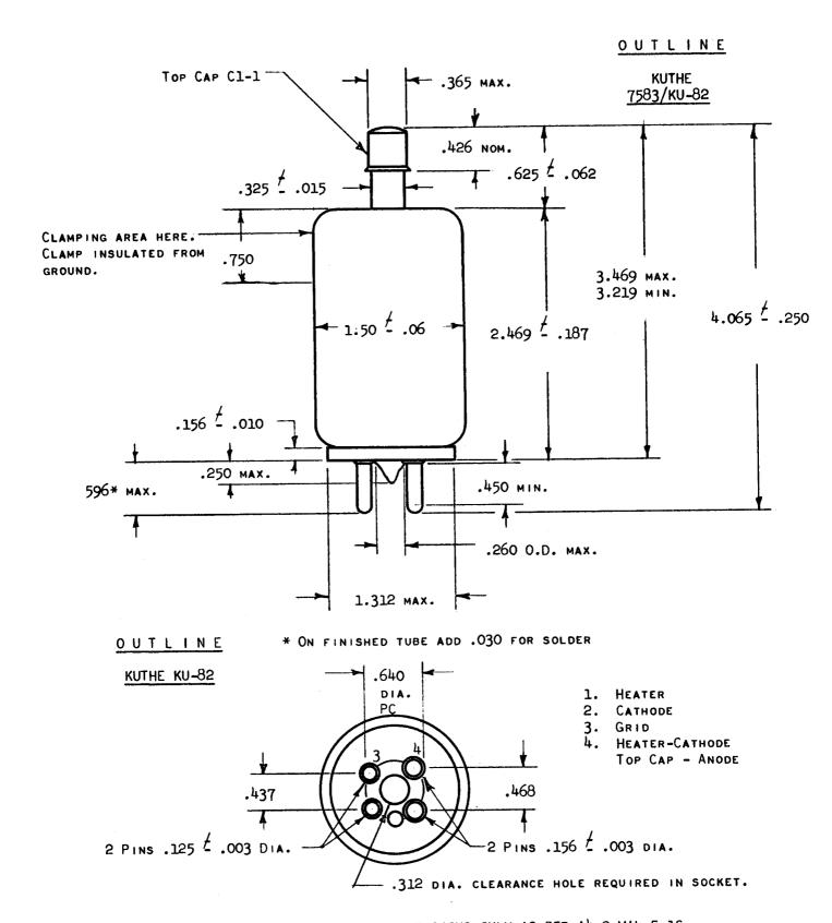
WAFER BASE. PIN ARRANGEMENT AND DIMENSIONS ONLY AS PER A4-9 MIL-E-1C
