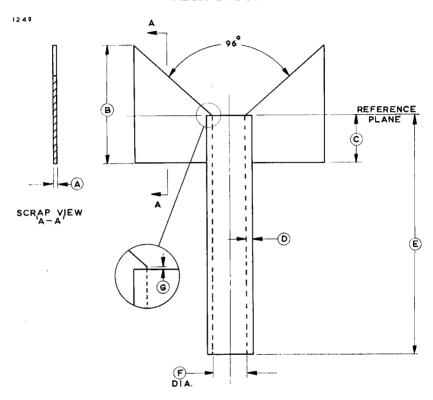
The gauge shown above will pass freely over base and neck to the reference line, and when rotated through  $360^{\circ}$  the blades of the gauge will contact the flared neck at the reference line only.
