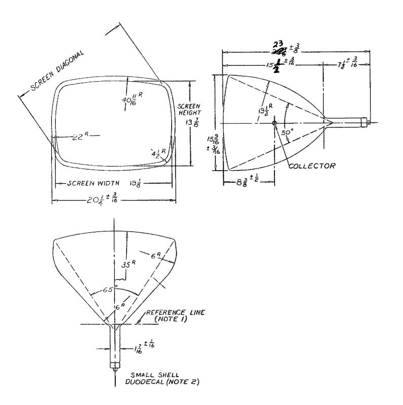
NOTE 1: With tube neck inserted through flared end of reference-line gauge (JETEC No. 110) and with tube seated in gauge, the reference line is determined by the inter-section of the plane CC' of the gauge with the glass funnel.
