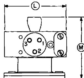
**NOTE:** Eyelet-type inserts in the flange mounting holes are 0.219 O.D., 0.185 I.D., nominal, and are easily removable from rear of flange. With inserts in place, the mounting holes provide clearance for #8 screws. With inserts removed, the mounting holes permit use of insulating bushings where d-c isolation between tube flange and waveguide system is desired.
