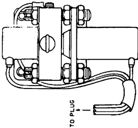
NOTE: Eyelet-type inserts in the flange mounting holes are 0.219 O. D., 0.185 I. D., nominal, and are easily removable from rear of flange. With inserts in place, the mounting holes provide clearance for #8 screws. With inserts removed, the mounting holes permit use of insulating bushings where d-c isolation between tube flange and waveguide system is desired.
