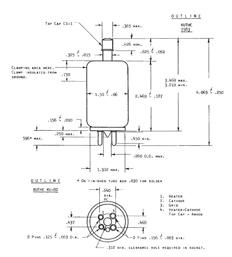
WAFER BASE. PIN ARRANGEMENT AND DIMENSIONS ONLY AS PER A4-9 MIL-E-10
