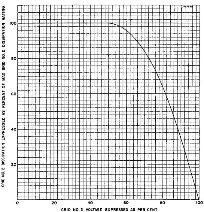
GRID NO.2 VOLTAGE EXPRESSED AS PER CENT OF MAX GRID NO.2 SUPPLY VOLTAGE RATING
